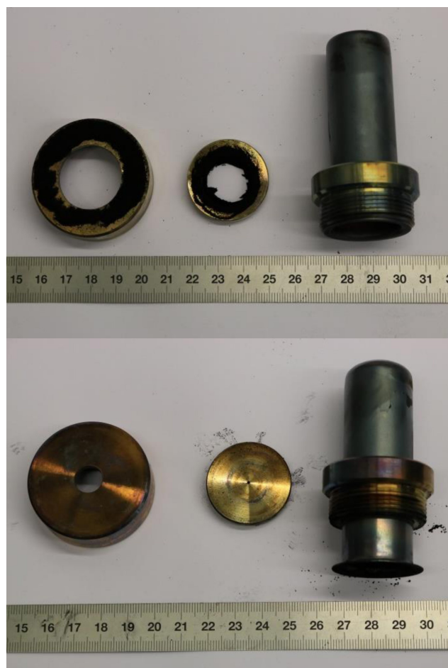
Figure 12. Steel tubes after testing with d40-HMTD. Top: 20 mm vent hole diameter of the orifice plate, the steel tube and the plate are still intact; bottom: 1 mm vent hole diameter; orifice plate and steel tube are both intact.
