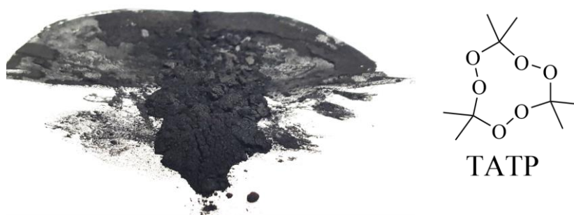
Figure 23. Left: phlegmatized activated charcoal-TATP mixture on a filter paper, right: structure of the TATP [5].
