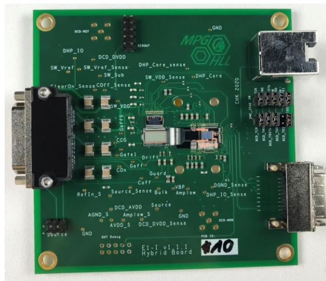
Figure 6-1: EDET Hybrid Board 1 (10 cm x 10 cm) with a small sensor of 128 x 64 pixels in the middle (flat grey surface 7.68 mm x 3.84 mm). North of it, one can find the Switcher chip, right to the matrix the DCDE and DHP. Various capacitors and resistors ensure stability for the different voltages. All supply voltages can be probed at the labeled access points. The board establishes its power connection by means of a 51 pole D-Sub-Micro-D Glenair connector at the left. The RJ45 connector provides the JTAG connectivity, whereas the Infiniband connector at the bottom right is responsible for the data transfer.
