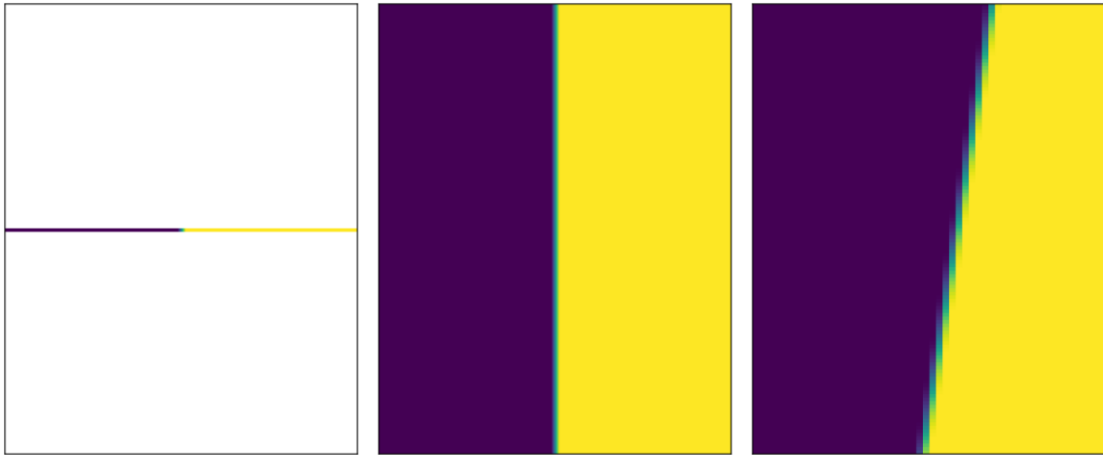
Figure 8-9: Simulated radioactive source on an EDET sensor with a slanted edge. Left: single line as outcome of the simulation process. Middle: repeat of the simulated line 128 times to reproduce the rows of an EDET small matrix. Right: tilt the edge transition region to an angle of 4.76^\circ .
