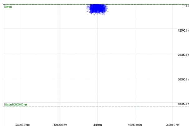
Figure 8-5: Monte Carlo Simulation of a 22 keV electron hitting a silicon layer with the same dimension as an EDET pixel. The blue heap on top symbolizes the different electron trajectories. The analysis was performed with 1,000 trajectories. Coordinates are in x and z direction and dimensions are given in nanometers.
