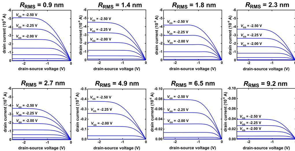
Figure S3. Measured output curves of the TFTs fabricated using gate dielectrics with different degrees of surface roughness.
