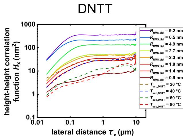
**Figure S7.** Calculated height-height correlation functions of DNTT films deposited onto gate dielectrics with different degrees of surface roughness (solid lines) and of DNTT films deposited onto a smooth gate dielectric but at different substrate temperatures during the DNTT deposition (dashed lines).
