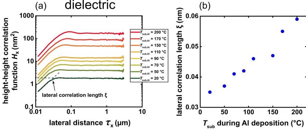
**Figure S6.** (a) Height-height correlation functions calculated along the fast scanning axis of the AFM of the surface of hybrid  $\text{AlO}_x/\text{SAM}$  gate dielectrics prepared on aluminum layers deposited at substrate temperatures ranging from 20 °C to 200 °C during the aluminum deposition. (b) Extracted lateral correlation lengths of the gate-dielectric surfaces as a function of the substrate temperature during the aluminum deposition.
