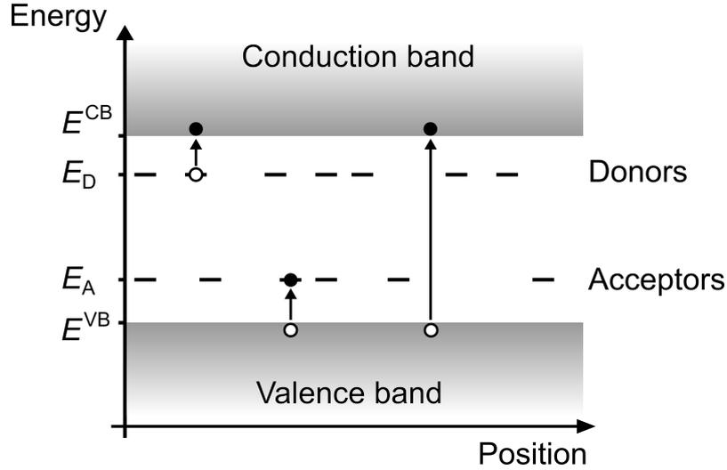
Figure 2.3: Band diagram of an extrinsic semiconductor. Discrete energy levels of donors, just below the conduction band, and acceptors, just above the valence band, can be ionized at room temperature and provide additional free charges.
