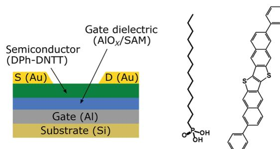
FIG. 1. Schematic cross section of the thin-film transistors with the thin gate dielectric, which consists of a 3.6-nm-thick layer of aluminum oxide ( $\text{AlO}_x$ ) and a 1.7-nm-thick self-assembled monolayer (SAM) of *n*-tetradecylphosphonic acid. The chemical structures of *n*-tetradecylphosphonic acid and of the organic semiconductor 2,9-diphenyl-dinaphtho[2,3-b:2',3'-f]thieno[3,2-b]thiophene (DPh-DNTT) are also shown.
