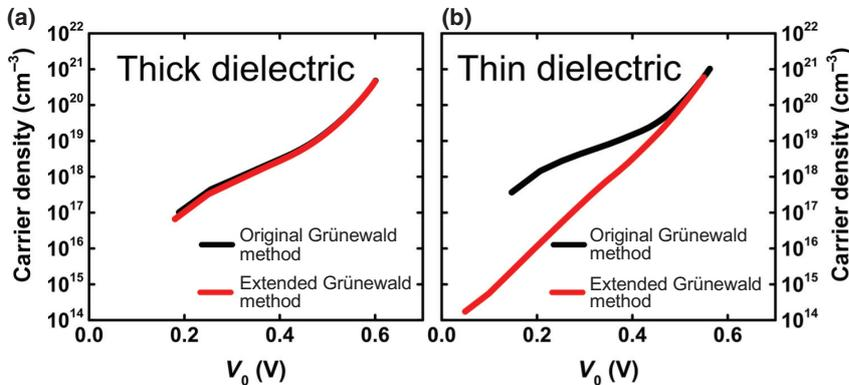
FIG. 6. Results of the second step of the Grünwald method in which the relation between the carrier density and the interface potential is calculated. This calculation is performed once using Eq. (9) (original method, shown with black lines) and once using Eq. (15) (extended method, shown with red lines).
