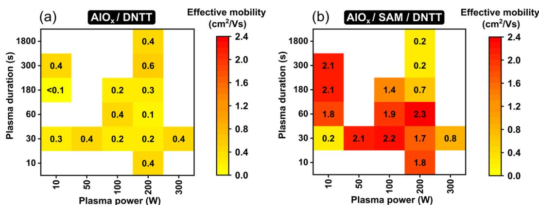
**Figure 6.** Effective charge-carrier mobilities extracted from the measured transfer characteristics of DNTT TFTs fabricated using either a bare- $\text{AlO}_x$  gate dielectric (a) or a hybrid  $\text{AlO}_x/\text{SAM}$  gate dielectric (b) as a function of plasma power and plasma duration.
