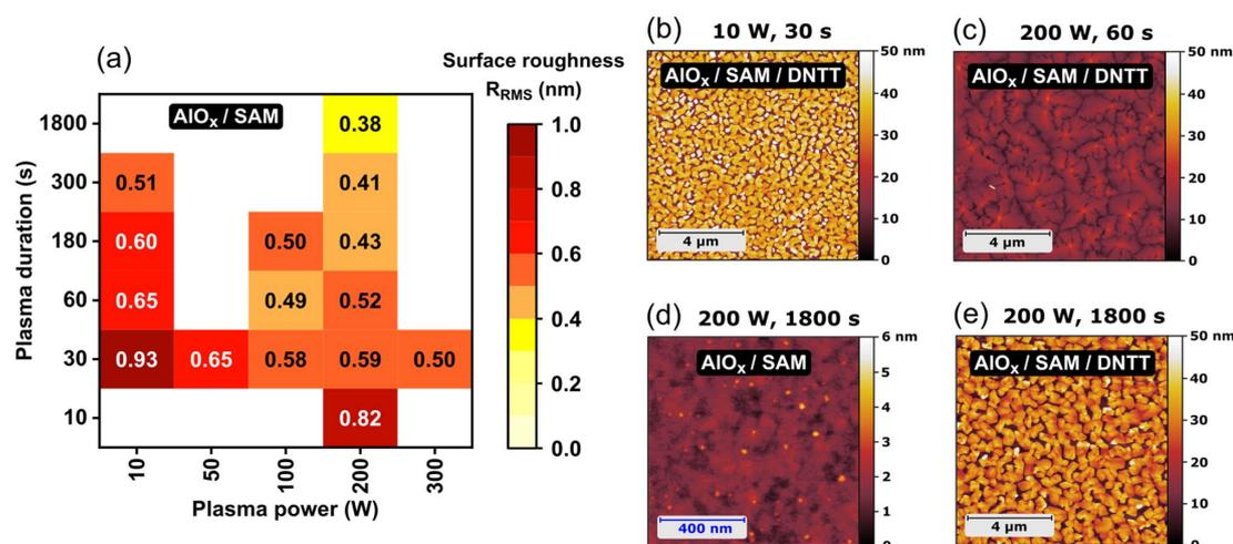
**Figure 8.** (a) Root-mean-square surface roughness of hybrid AIO<sub>x</sub>/SAM dielectrics as a function of plasma power and plasma duration. (b–e) AFM images of representative morphologies on the indicated surfaces with the indicated plasma parameters.
