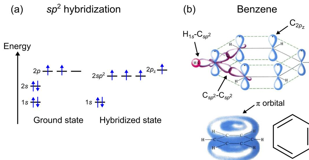
Figure 2.7: (a) Energetic structure of a carbon atom in its ground state and in the  $sp^2$  hybridization. The 2s orbital and two 2p orbitals hybridize and form three degenerated  $2sp^2$  orbitals. (b) Atomic orbitals of the individual atoms in a benzene molecule. The  $2p_z$  atom orbitals of the six carbon atoms hybridize and form a delocalized  $\pi$  orbital. Adapted from reference 39.
