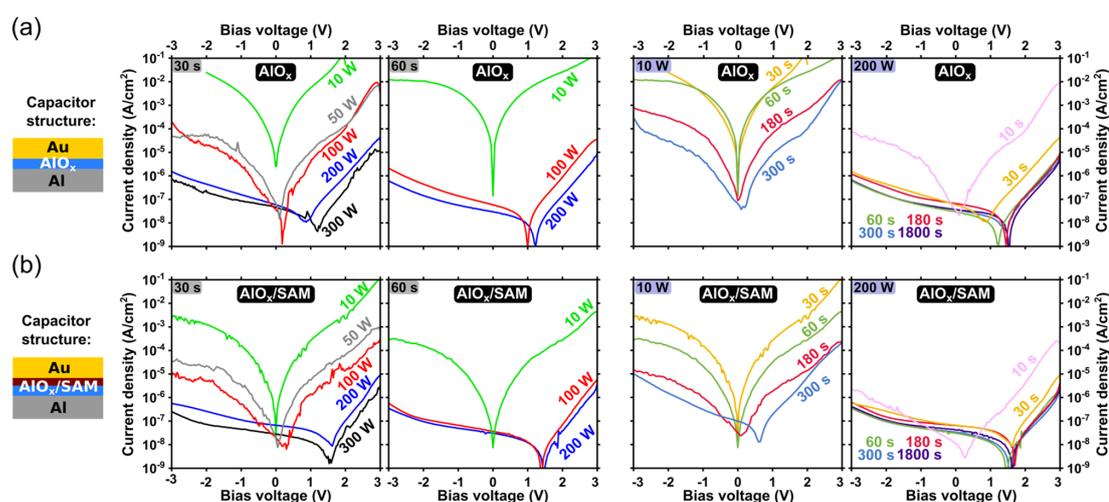
**Figure 4.** Current density measured as a function of applied voltage through capacitors with a bare-AIO<sub>x</sub> dielectric (a) and a hybrid AIO<sub>x</sub>/SAM dielectric (b) for various combinations of plasma power and plasma duration.
