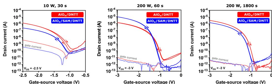
**Figure 5.** Transfer characteristics and gate currents of DNTT TFTs fabricated using either a bare- $\text{AlO}_x$  gate dielectric (red curves) or a hybrid  $\text{AlO}_x/\text{SAM}$  gate dielectric (blue curves) for three combinations of plasma power and plasma duration. (Fig. S3 shows the complete set of results.) The TFTs have a channel length of  $20\ \mu\text{m}$  and a channel width of  $100\ \mu\text{m}$ .
