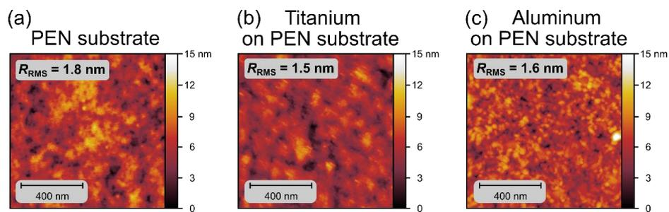
**Figure S1.** Atomic force microscopy (AFM) images and root-mean-square surface roughness of (a) the surface of a PEN substrate, (b) a 25-nm-thick vacuum-deposited titanium film on PEN, and (c) a 25-nm-thick vacuum-deposited aluminum film on PEN.
