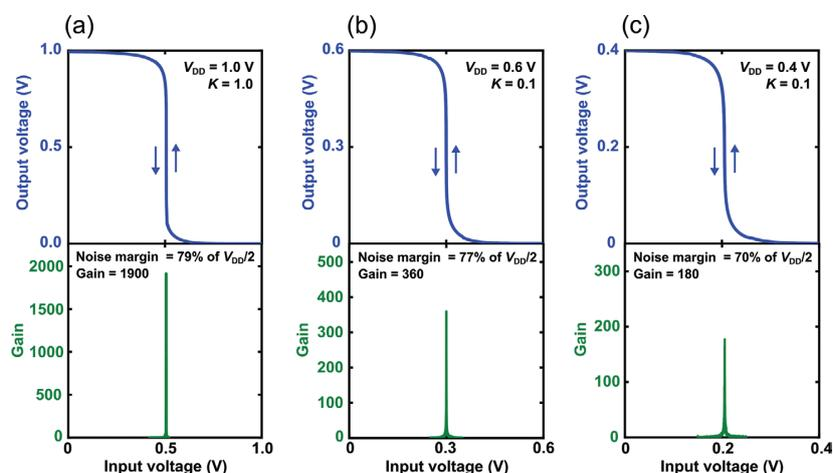
**Figure 8.** Measured transfer characteristics of zero- $V_{GS}$  inverters based on DPh-DNTT TFTs with Ti/TiO<sub>x</sub>/SAM and Al/AlO<sub>x</sub>/SAM gate stacks for the load and drive TFTs, respectively.
