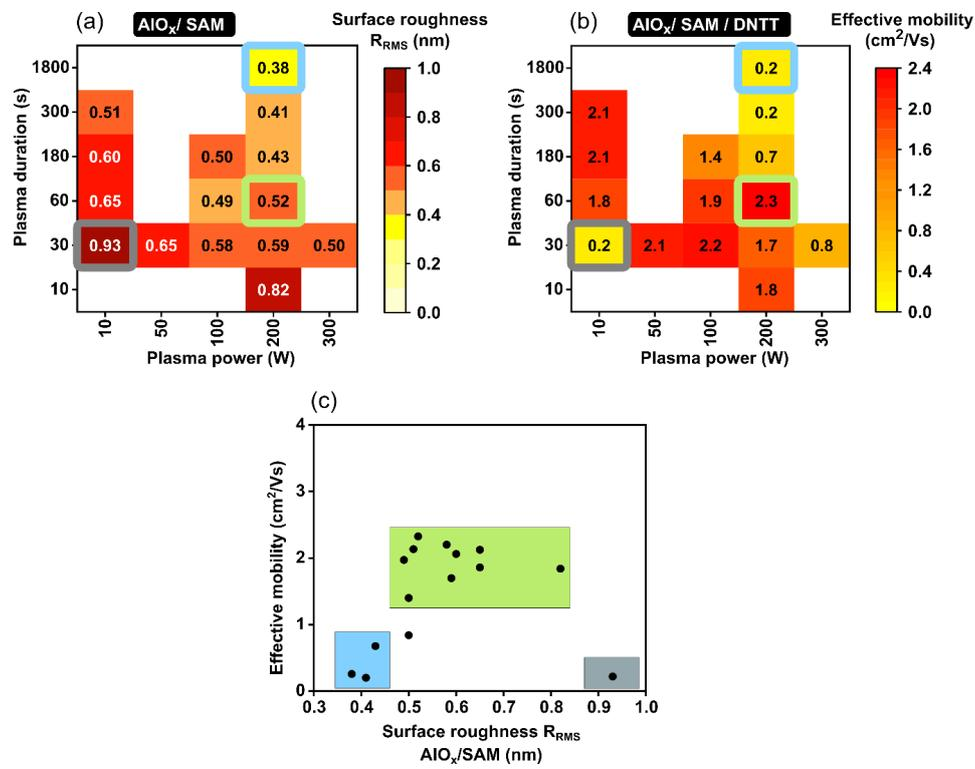
Figure S5: (a) Root-mean-square surface roughness of hybrid  $AIO_x/SAM$  dielectrics as a function of plasma power and plasma duration. (b) Carrier mobilities extracted from the measured transfer characteristics of DNTT TFTs fabricated using a hybrid  $AIO_x/SAM$  gate dielectric as a function of plasma power and plasma duration. (c) Carrier mobility plotted as a function of the RMS surface roughness.
