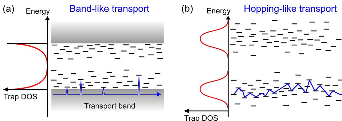
Figure 2.9: (a) Illustration of the transport mechanism for a band-like transport. Charge carriers frequently get trapped in localized states and are thermally released again. In an extended transport band, charge transport is possible. (b) Illustration of hopping-like transport. There are no electronic bands, but charge carriers can hop from one localized state to another by phonon-assisted tunneling.
