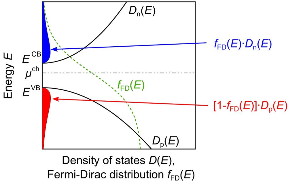
Figure 2.2: Density-of-states functions for electrons  $D_n$  and holes  $D_p$  and the Fermi-Dirac distribution function  $f_{\text{FD}}$  for  $T > 0\text{ K}$ . The density of electrons which are excited into the conduction band is represented as blue area, the density of holes in the valence band is represented as red area. Due to charge neutrality both areas have to be equal and the chemical potential  $\mu^{\text{ch}}$  adjusts accordingly. Adapted from reference 29.
