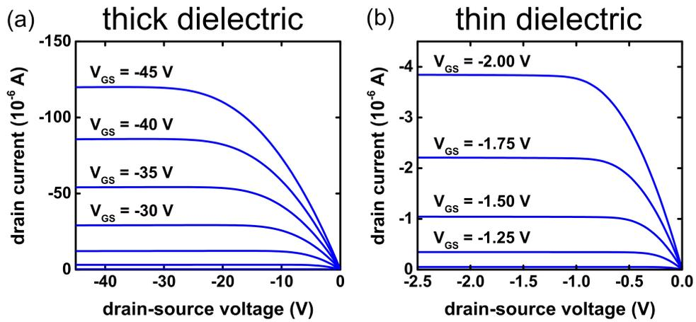
FIG. S1. Measured output characteristics of the transistors with the 110-nm-thick gate dielectric (a) and the 5.3-nm-thick gate dielectric (b).
