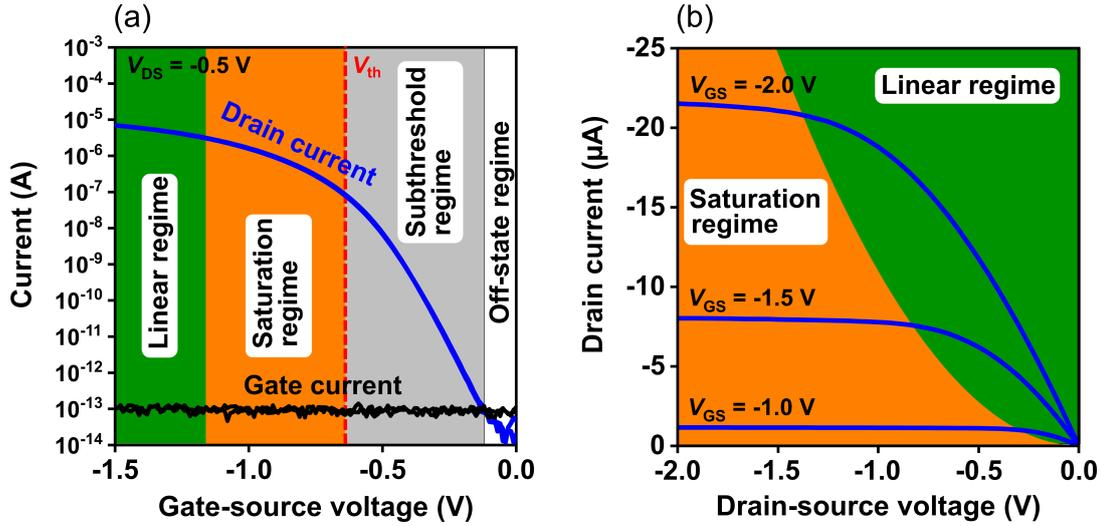
Figure 2.6: (a) Transfer characteristic and (b) output characteristic of a p-channel organic TFT. The different regimes of operation are highlighted.
