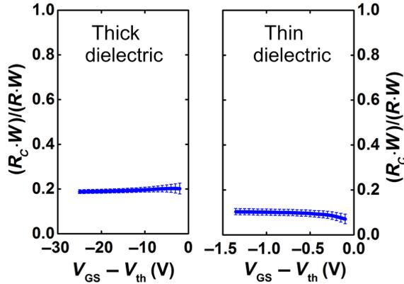
FIG. 8. Ratio between the channel-width-normalized contact resistance ( $R_C \cdot W$ ) and the channel-width-normalized total device resistance ( $R \cdot W$ ) for TFTs with a channel length of  $100 \mu\text{m}$ , measured using the transmission line method (TLM) and plotted as a function of the difference between the gate-source voltage and the threshold voltage. For both types of TFT (thick and thin gate dielectrics), the contact resistance is small compared to the total resistance.
