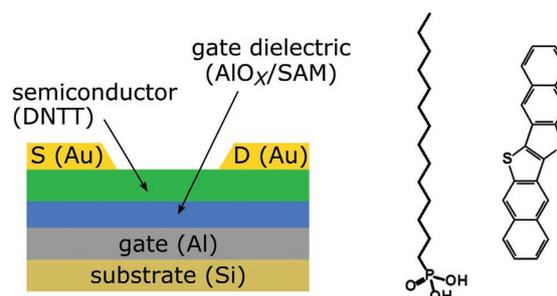
**Figure 1.** Schematic cross-section of the organic TFTs and chemical structures of *n*-tetradecylphosphonic acid for the gate-dielectric SAM and the organic semiconductor dinaphtho[2,3-b:2',3'-f]thieno[3,2-b]thiophene (DNTT).
