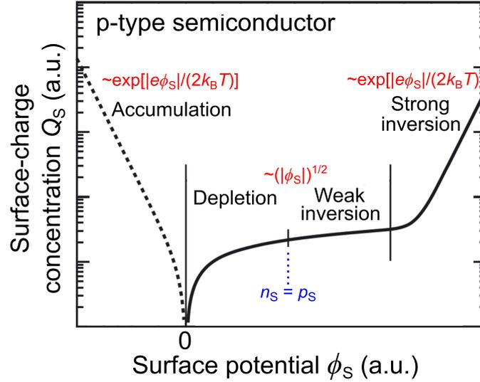
Figure 2.4: Surface-charge concentration of a p-type semiconductor plotted as a function of the surface potential. For the different regimes of operation, the dominant term contributing to the surface charge is given. For the accumulation regime, the surface charge has an exponential dependence on the surface potential and can be varied by orders of magnitude. Adapted from reference 36.
