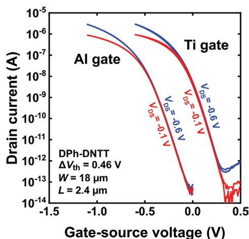
**Figure 6.** Measured transfer characteristics of flexible DPh-DNTT TFTs with an Al/AlO<sub>x</sub>/SAM gate stack (left) and a Ti/TiO<sub>x</sub>/SAM gate stack (right). The TFTs with the Al/AlO<sub>x</sub>/SAM gate stack have a negative turn-on voltage, while the TFTs with the Ti/TiO<sub>x</sub>/SAM gate stack have a positive turn-on voltage. The difference between the threshold voltages is 0.46 V.
