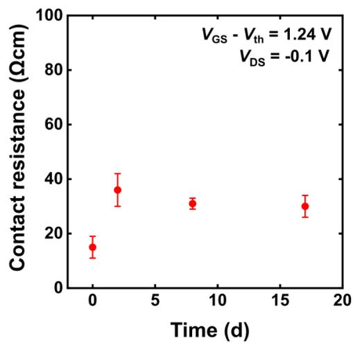
**Figure S3.** Evolution of the width-normalized contact resistance of flexible DPh-DNTT TFTs with a Ti/TiO<sub>x</sub>/SAM gate stack over a period of 17 days after fabrication while being stored in ambient air with a relative humidity of about 40%.
