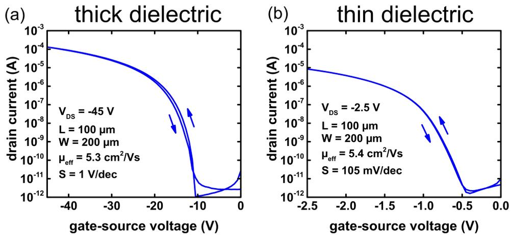
FIG. S2. Transfer curves measured on the TFTs with a 110-nm-thick gate dielectric (a) and a 5.3-nm-thick gate dielectric (b). The transfer curves were measured in the saturation regime of operation.
