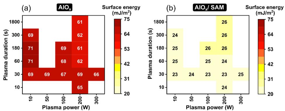
Figure S7: Surface energy of bare-AIO<sub>x</sub> dielectrics (a) and hybrid AIO<sub>x</sub>/SAM dielectrics as a function of plasma power and plasma duration.
