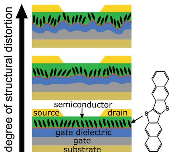
**Figure 4.** A rough gate electrode correlates with a rough gate dielectric and introduces structural distortion in the semiconductor film. This structural distortion, represented mainly by grain boundaries and their density, leads to the formation of transport barriers and trap states that have a detrimental effect on the electric characteristics of the TFTs.
