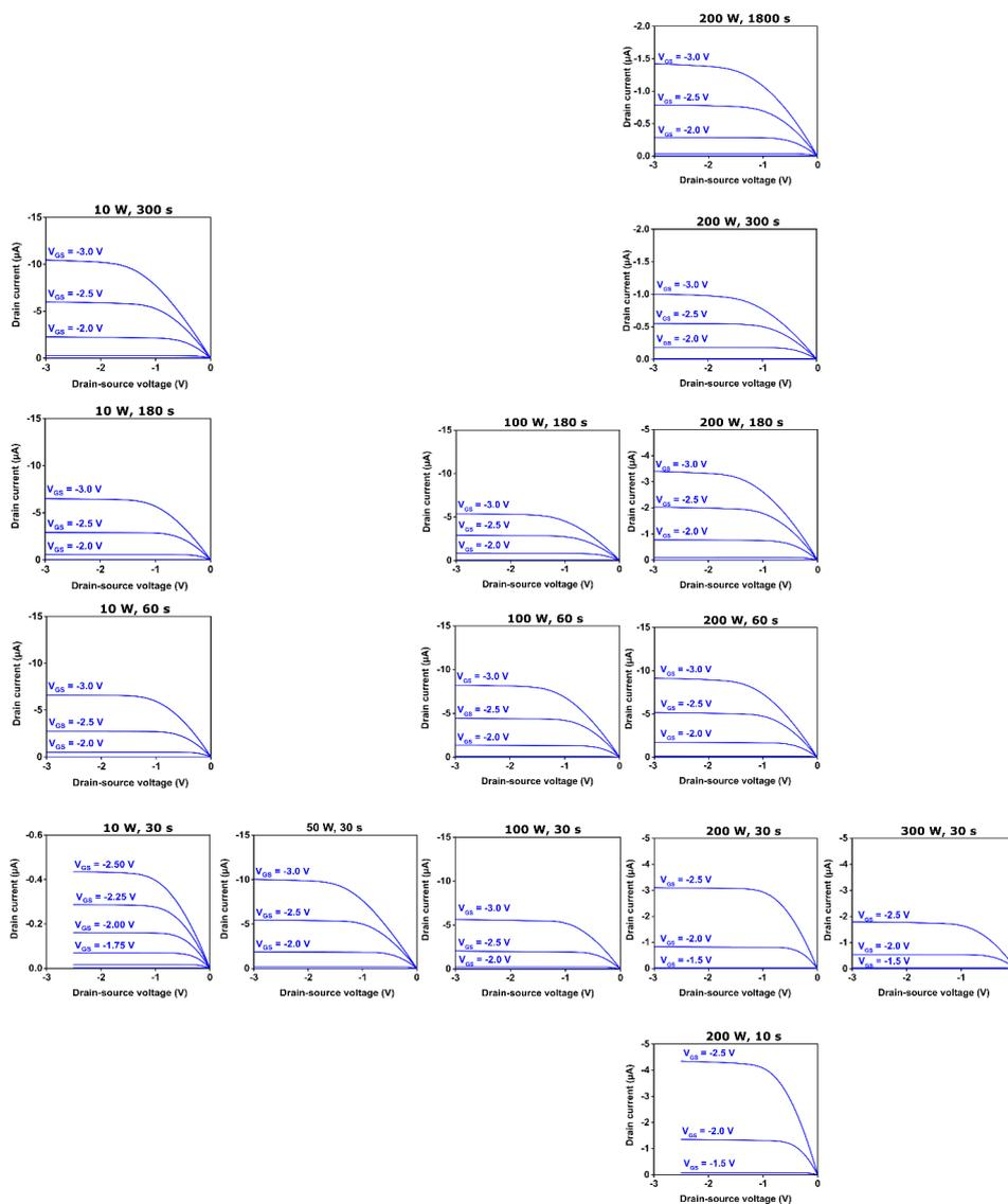
Figure S4: Output characteristics of DNTT TFTs fabricated using a hybrid  $\text{AlO}_x/\text{SAM}$  gate dielectric for all fifteen combinations of plasma power and plasma duration.
