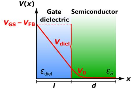
FIG. 4. Sketch of the potential drop across the gate dielectric and the semiconductor layer of the transistor. In the original Grünwald method, it is assumed that  $|V_0| \ll |V_{GS}|$  and, hence,  $V_0$  is ignored. In the extended Grünwald method proposed here, this simplification is removed, and the contribution of  $V_0$  is correctly taken into account.
