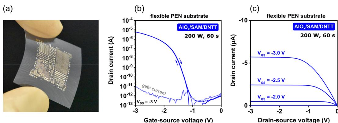
**Figure 9.** (a) Photograph of organic TFTs and circuits fabricated on a flexible polyethylene naphthalte (PEN) substrate. (b) Measured transfer and (c) output characteristics of a DNTT TFT with a channel length of 20  $\mu\text{m}$  and a channel width of 100  $\mu\text{m}$  on flexible PEN. The effective charge-carrier mobility is 2  $\text{cm}^2/\text{Vs}$ .
