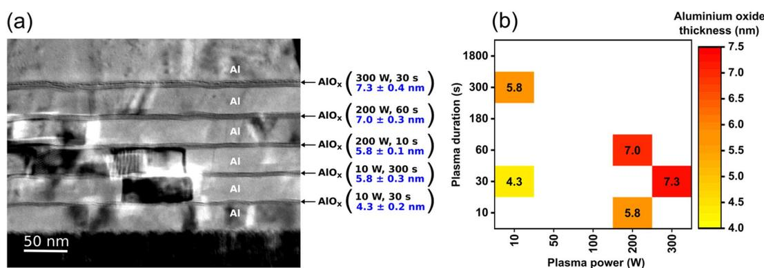
**Figure 1.** Thickness of plasma-grown aluminum oxide films. (a) Cross-sectional TEM image indicating the thicknesses of five AlO<sub>x</sub> films produced sequentially by the plasma-assisted surface oxidation of aluminum using five different combinations of plasma power and plasma duration. (b) Summary of the results.
