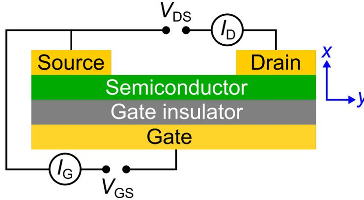
Figure 2.5: Schematic cross-section of a field-effect transistor. Please note the convention used in this chapter: The  $x$ -direction is perpendicular and the  $y$ -direction is parallel to the insulator/semiconductor interface.
