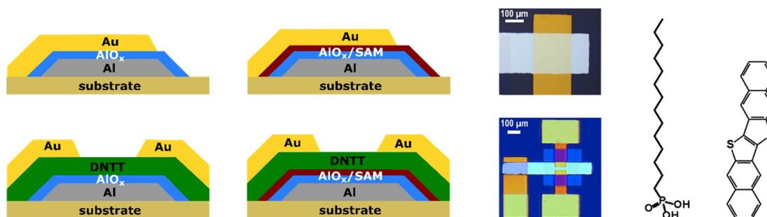
**Figure 2.** Schematic cross sections and photographs of metal–insulator–metal capacitors and bottom-gate, top-contact TFTs in which the insulator or gate dielectric is either a film of plasma-grown  $\text{AlO}_x$  or a combination of plasma-grown  $\text{AlO}_x$  and an *n*-tetradecylphosphonic acid SAM. Also shown are the chemical structure of *n*-tetradecylphosphonic acid and of the organic semiconductor dinaphtho[2,3-*b*:2',3'-*f*]thieno[3,2-*b*]thiophene (DNTT).
