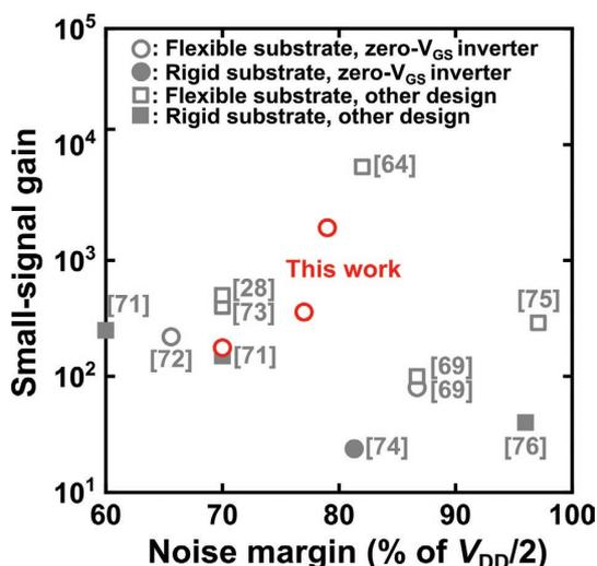
**Figure 9.** Literature summary of organic-TFT-based unipolar inverters with a small-signal gain of at least 10 and a noise margin of at least 60% of half the supply voltage.
