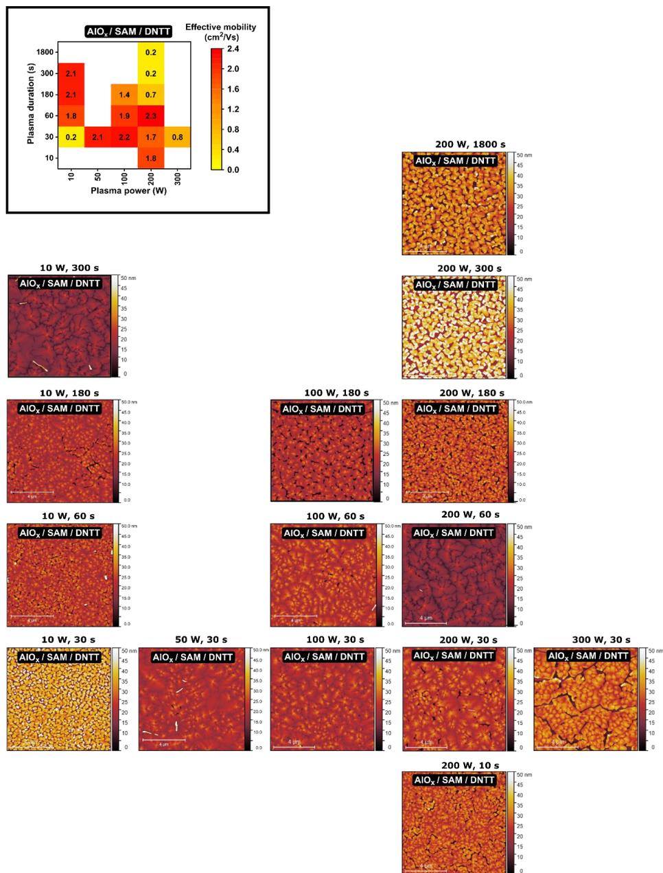
Figure S6: AFM images of DNTT films deposited onto hybrid  $\text{AlO}_x/\text{SAM}$  dielectrics for all fifteen combinations of plasma power and plasma duration.
