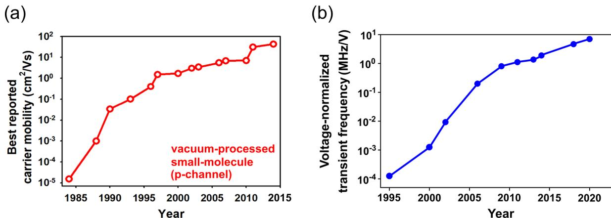
Figure 1.1: (a) Evolution of the charge-carrier mobility of organic small-molecule semiconductors deduced from field-effect transistor (FET) measurements. Adapted from references 5 and 6. (b) Literature overview of the highest voltage-normalized transit frequencies of organic TFTs over time. This value characterizes the dynamic performance of TFTs and is essential for most electronic applications. Adapted from reference 7.
