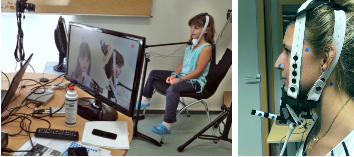
Fig. 5. Ultrasound recording set-up in the first year of recordings on the left and the probe-holder system used in the second year of recordings on the right.
