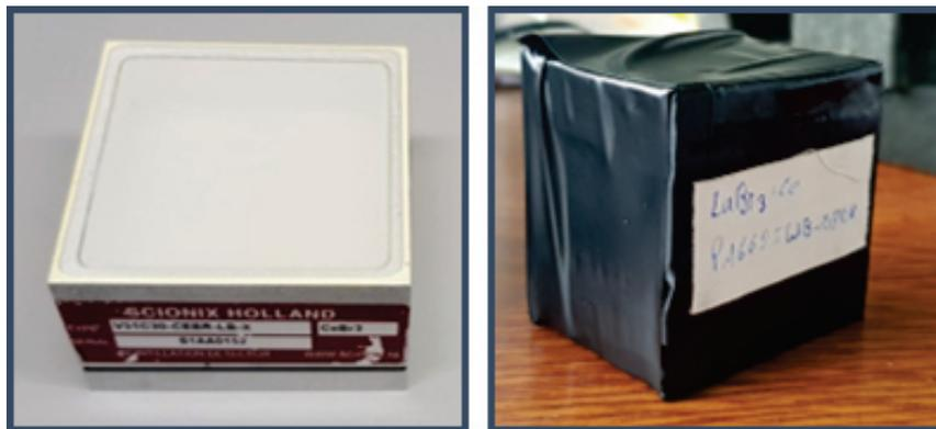
**Fig. 6.15:** Picture of one of the monolithic  $\text{CeBr}_3$  crystals (left) and of the coupled absorber detector (here:  $\text{LaBr}_3:\text{Ce}$  and PA6625WB-0808) including black tape wrapping (right).
