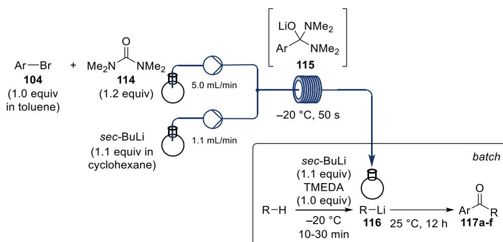
**Scheme 26:** Continuous flow reaction set-up for the preparation of unsymmetrical ketones of type **117** by the stepwise acylation of TMU (**114**) with different lithium organometallics.
