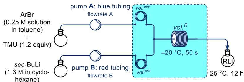
**Scheme 38:** Flow chemistry setup for preparation of unsymmetrical ketones starting from TMU, aryl bromides and *sec*-BuLi in a Barbier-type reaction.
