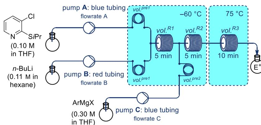
**Scheme 39:** Flow chemistry setup for preparation highly functionalized ketones.
