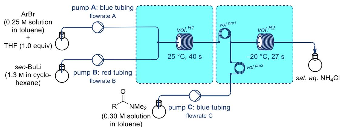
**Scheme 37:** Flow chemistry setup for preparation of ketones starting from lithium species, prepared via Br/Li exchange in flow, and *N,N*-dimethylamides.
