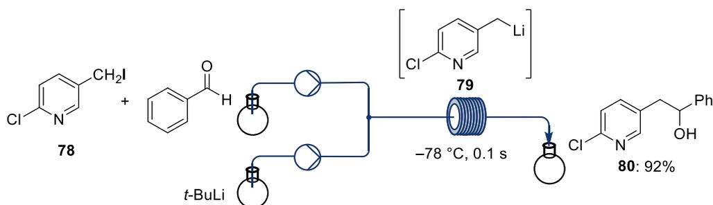
**Scheme 16:** Preparation and consumption of benzylic lithium species in a Barbier-type continuous flow set-up.
