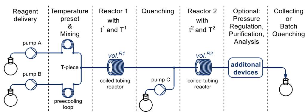
**Figure 2:** General 3-pump continuous flow setup of a 2-step procedure.
