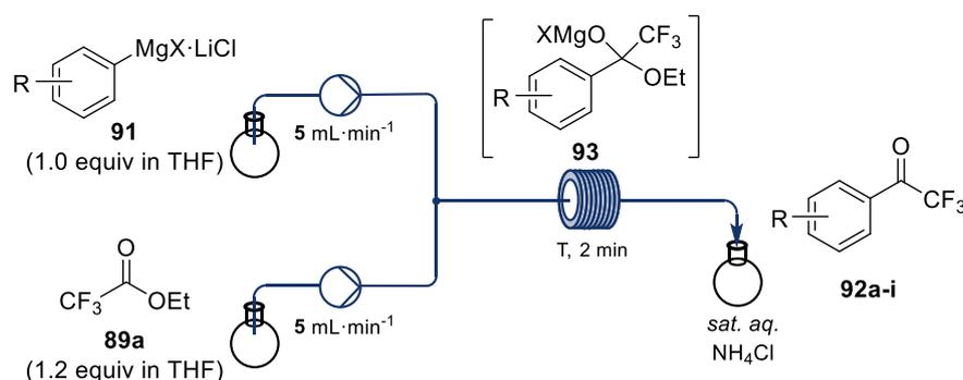
**Scheme 23:** Continuous flow setup for the preparation of trifluoromethyl ketones of type **92**.
