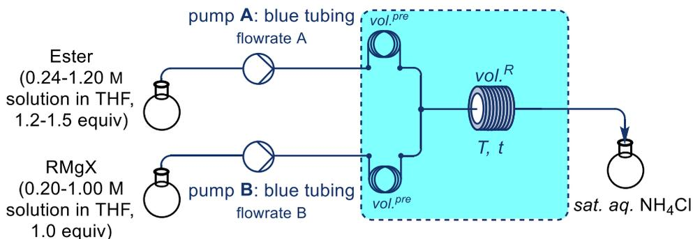
**Scheme 36:** Flow chemistry setup for preparation of ketones starting from Grignard reagents and esters.
