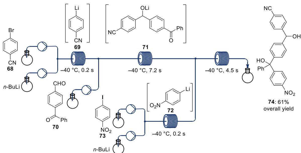
**Scheme 14:** Chemoselective halogen/Li exchanges in a multi-step continuous flow set-up for the preparation of the highly functionalized compound **74**.
