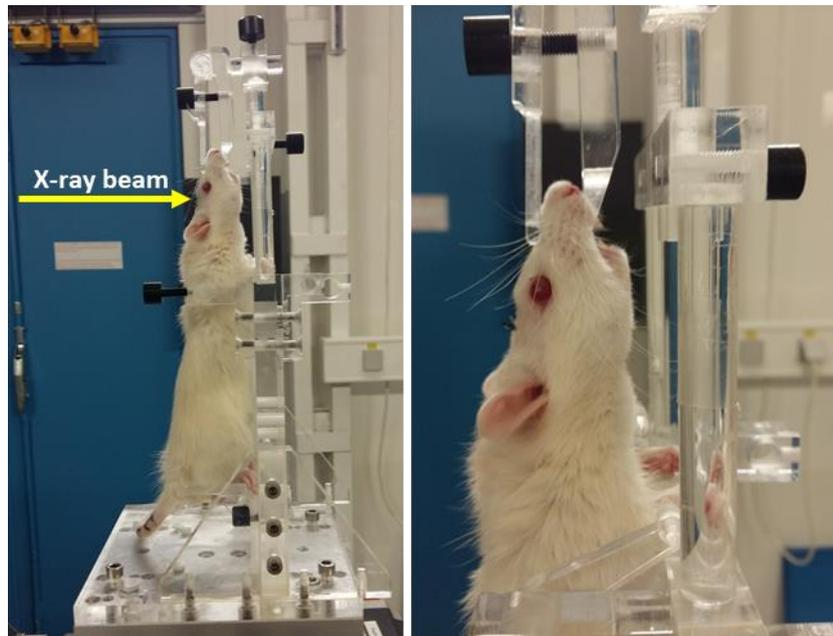
Figure 3.6: rat positioning for the MRT irradiation in the EH1 of the ID17 beamline. The X-ray beam path is identified by the yellow arrow that points at the RT target which is, in this case, the right brain hemisphere. The zoomed picture shows how the rat head is blocked.
