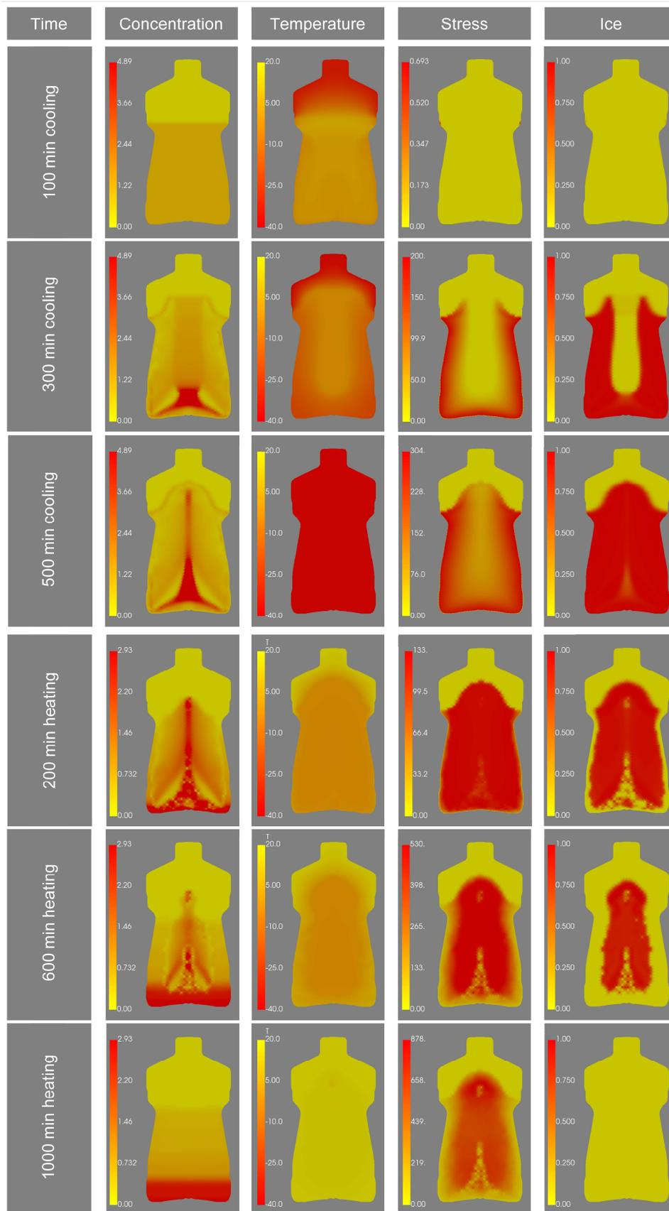
**Figure 6** Simulated development of mAb concentration (CF), temperature (°C), local stress, and the formation of ice during cooling and heating.
