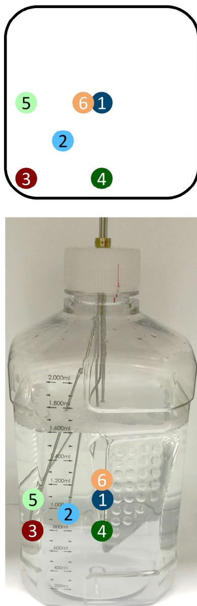
**Figure 1** Positioning of TCs in the 2 L PharmaTainer™ bottle. On top a schematic drawing in cross-section is provided, below a representative picture of the bottle. The figure is adapted from Bluemel et al. (2).
