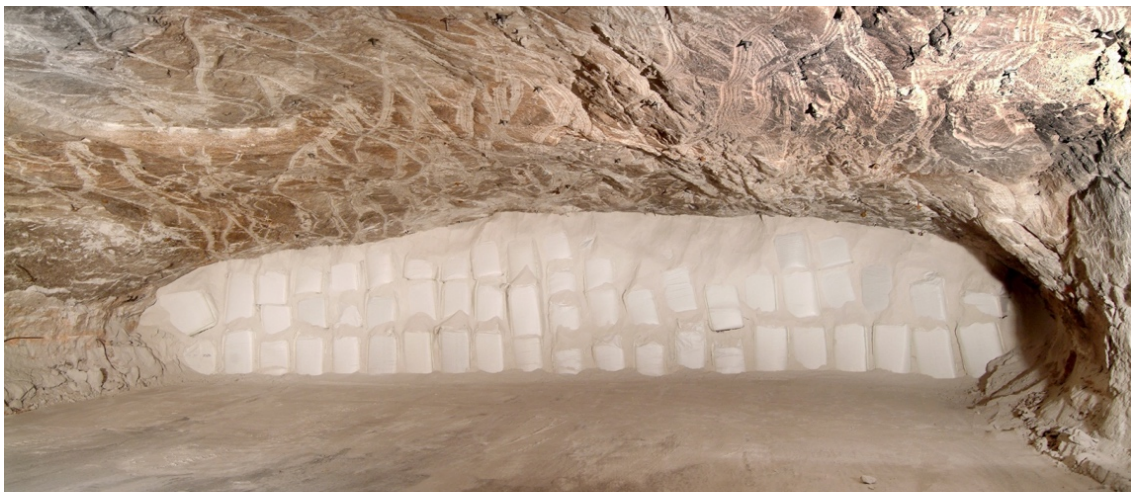
Figure 2.4: Utilization of FGT residues stored in big bags for stabilization in parts of salt mines where backfilling is required.
