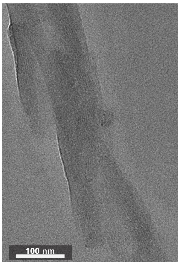
Figure 5-13: High resolution TEM image of PDI-MOF-74(Zn) in side view, showing a close-up of the lattice planes as inset.
