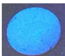
Figure 3-15: Photo image of an ANMOF-74(Mg) pellet during irradiation with a 365 nm wavelength.
