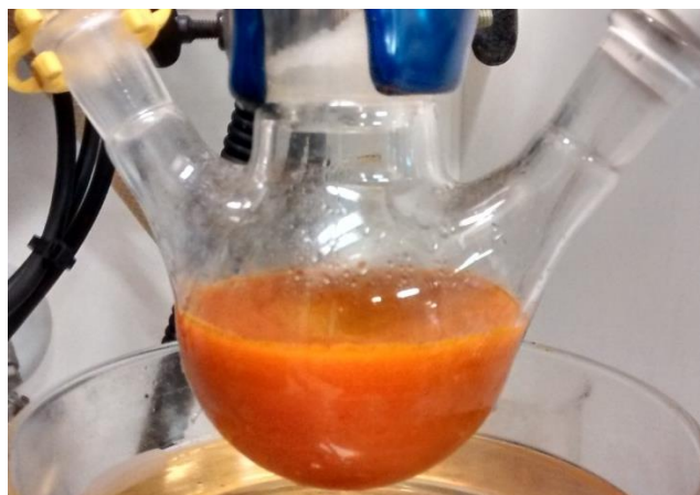
Figure S 6.1 Crude product. Reaction vessel showing the bright orange product right before filtering it off.
