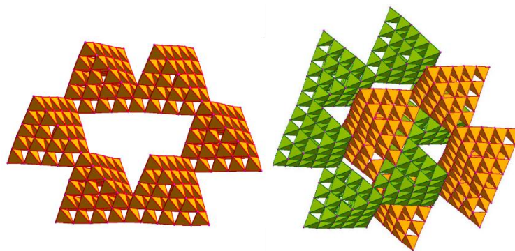
Figure S21: Six-membered ring motive of all-fused T5 supertetrahedra the whole structure can be described with in HT- \text{NaSi}_2\text{P}_3 (left). Only one single interpenetration mode is existent (right).
