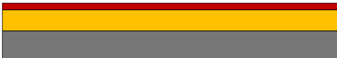
Figure 18: Schematic of the rotigotine transdermal therapeutic system; with backing foil (red), API-loaded adhesive matrix (orange) and release liner (grey)
