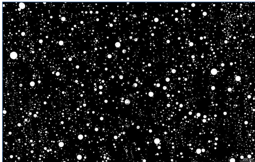
Figure 31: Stepwise treatment of the micro-CT images: Raw image of the chosen ROI (top); image after thresholding (middle); image after thresholding and the removal of stray particles (bottom).
