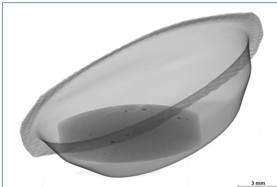
Figure 2: Radiograph of a pharmaceutical tablet sealed in a blister cup.
