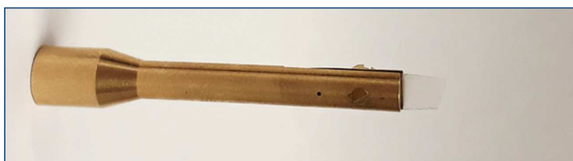
Figure 28: Patch cutout mounted on a precision clamp sample holder.
