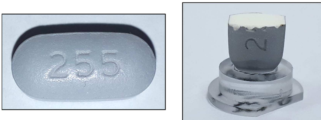
Figure 15: Sample tablet (left) and the same tablet after sample preparation for Raman microscopy.
