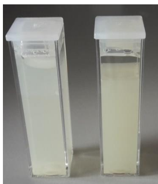
Figure S3.48: Images of suspensions, which were allowed to stand for 2 h with MeOH (left) and TEoA (right). After these 2 hours, sedimentation of particles in the MeOH containing sample can be observed, which is the reason for measuring smaller particles sizes within the suspension.
