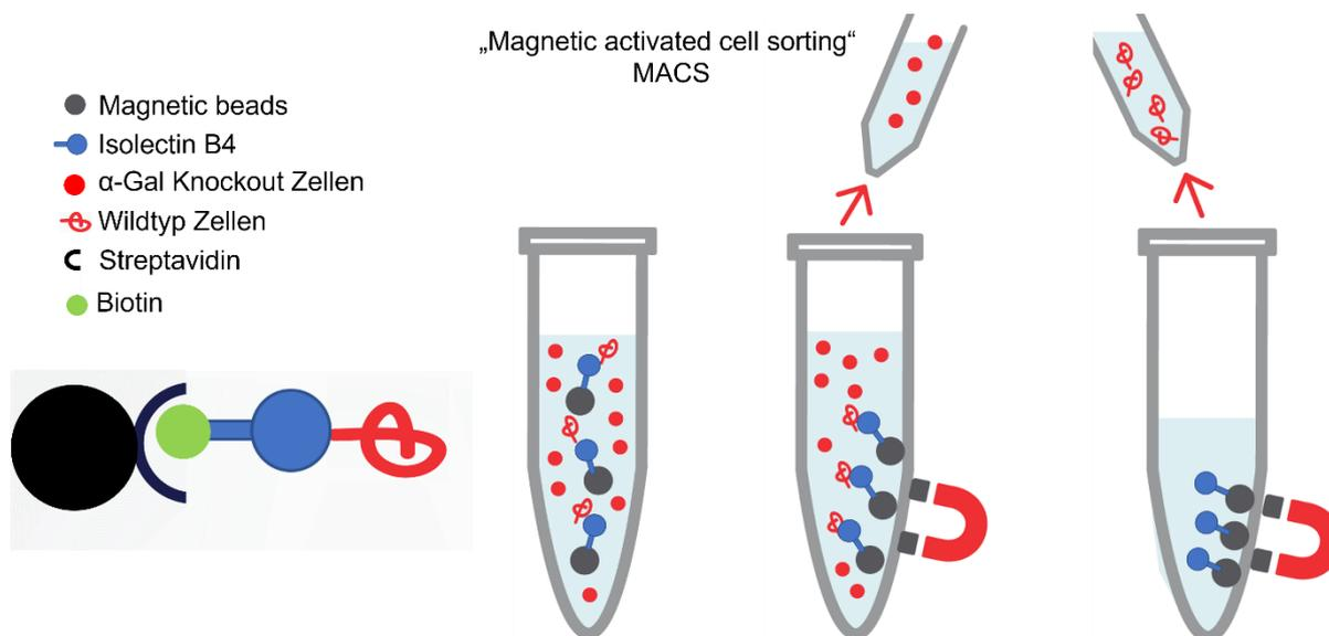
**Figure 7:** Separation of  $\alpha$ -Gal positive and negative cells by magnetic-activated cell sorting. Streptavidin coated magnetic beads bind to the biotinylated isolectin B4. A magnetic field is applied, and the  $\alpha$ -Gal negative cells are removed whereas the  $\alpha$ -Gal positive cells remain bound to the magnetic beads.
