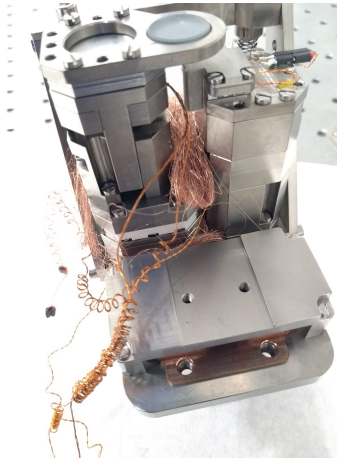
Figure 5.22.: Copper wool is added between the two stacks of the cavity setup to introduce a friction-based differential motion reduction.
