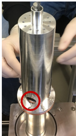
Figure 3.5.: Original design of shield for the cold head with four round apertures (circa 2 cm diameter) at the base (highlighted in red) for efficient pumping.
