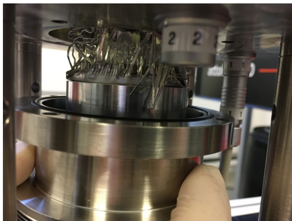
Figure 3.1.: A picture of broken 40 K link. The visual confirmation of fragile thermal link connecting the first stage of cold head to the cold shield on optical table was broken.
