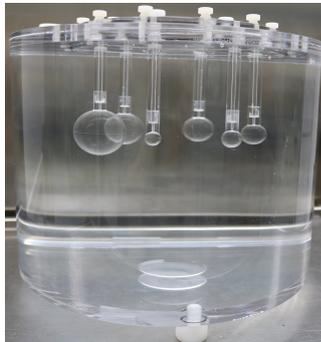
Figure 3.4: NEMA IEC Body Phantom Set<sup>TM</sup>.
