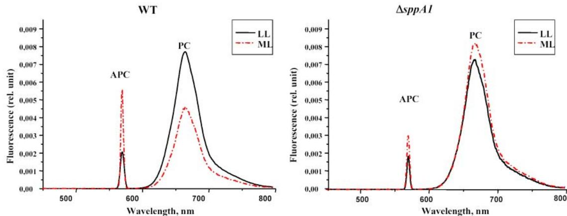
**Figure 31. Fluorescence excitation spectra at room temperature (25°C) of phycobilisomes extracted from wild-type and  $\Delta$ *sppA1* mutant grown under LL or ML.** Intact PBS of both strains were isolated with sucrose gradients by ultracentrifugation, concentrated and resuspended in 0.6 M phosphate buffer. PBS were incubated for 15 min at room temperature for partial dissociation. The excitation spectra were collected at an emission at 695 nm.
