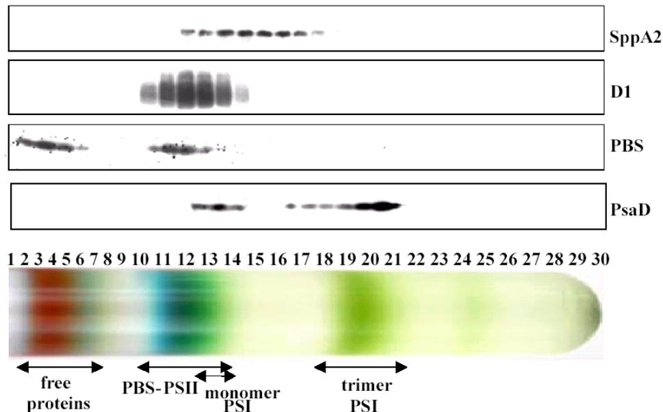
**Figure 39. Isolation of photosynthetic complexes from wild-type *Synechocystis* cells on sucrose gradients.** Thylakoid membranes from wild-type were solubilized with 2% of n-dodecyl- $\beta$ -D-maltoside and separated on a linear 12 to 24% MOPS-containing sucrose gradient. Fractions of 0.3-ml were collected for analysis of photosynthetic complexes and SppA2 using antisera directed against SppA2, D1 (PSII), PsaD (PSI) and phycocyanin proteins of phycobilisome rods.
