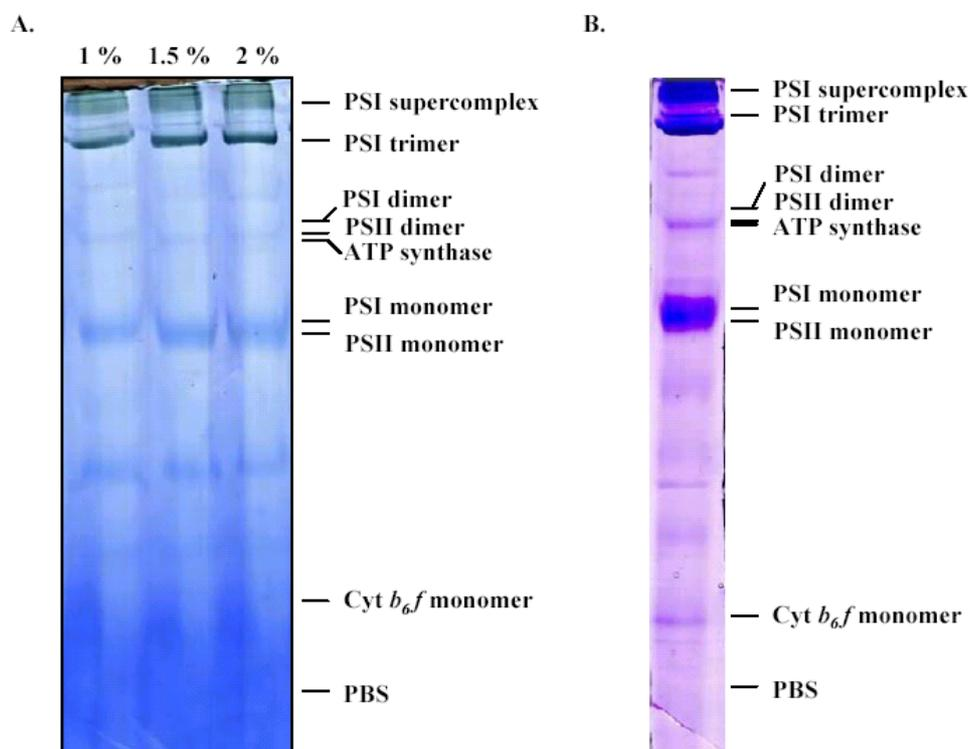
**Figure 40. Isolation of photosynthetic complexes from wild-type *Synechocystis* cells by non-denaturing 4 – 12% „blue native” gel electrophoresis. (A)** Thylakoids from the wild-type were solubilized with different concentrations of n-dodecyl- $\beta$ -D-maltoside (1, 1.5 and 2%) and used for isolation of major photosynthetic complexes by non-denaturing “blue native” gel electrophoresis. **(B)** Protein complexes were visualized by Coomassie Blue staining.
