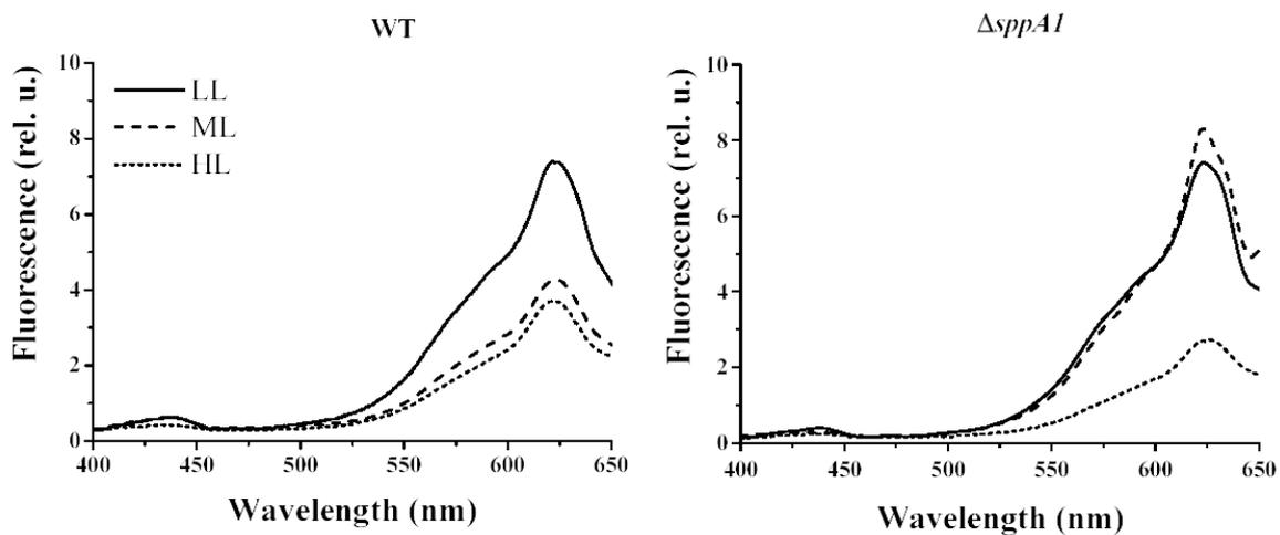
**Figure 22. Low-temperature (77 K) fluorescence excitation spectra of wild-type and  $\Delta sppA1$  strain at LL, ML and HL regimes.** *Synechocystis* cells of wild-type and  $\Delta sppA1$  were grown and adapted to ML and HL for 36 h. The excitation spectra were recorded at emission of 695 nm.
