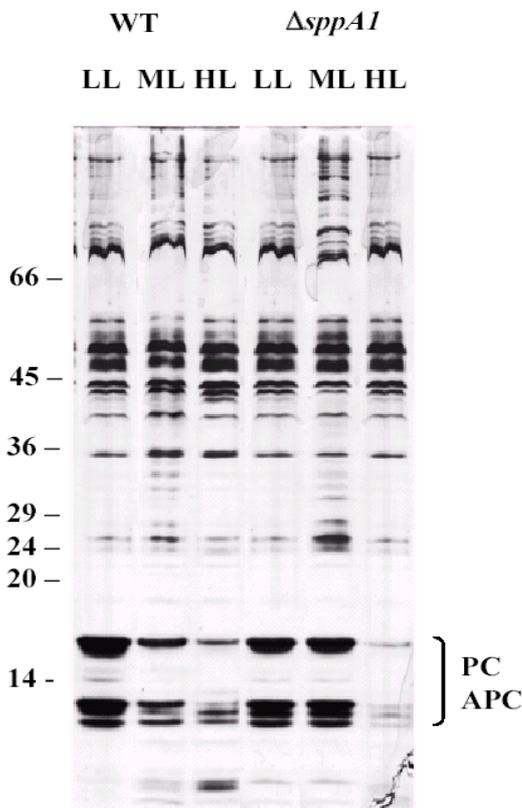
**Figure 24. Separation of thylakoid membrane proteins from *Synechocystis* wild-type and  $\Delta sppA1$  mutant.** Thylakoid proteins were isolated from cyanobacterial cells adapted for 3 days to LL, ML or HL regimes and separated by 12% SDS-PAGE. The proteins were visualized by silver staining. The positions of phycobiliproteins (PC and APC) are indicated by a bracket.
