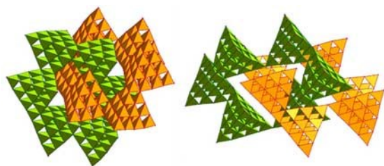
Figure B15 Two different interpenetration modes of symmetrically equivalent networks in \text{Na}_{23}\text{Si}_{37}\text{P}_{57} . Ring a is interpenetrated by ring b (left) and a homo-interpenetration of ring b can be observed (right).
