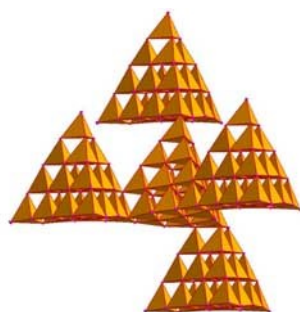
Figure B13 Supertetrahedral building unit of \text{Na}_{23}\text{Si}_{37}\text{P}_{57} . A T4 cluster is fused with three other T4 entities by one common \text{SiP}_4 unit and vertex shared with another T4 supertetrahedron.
