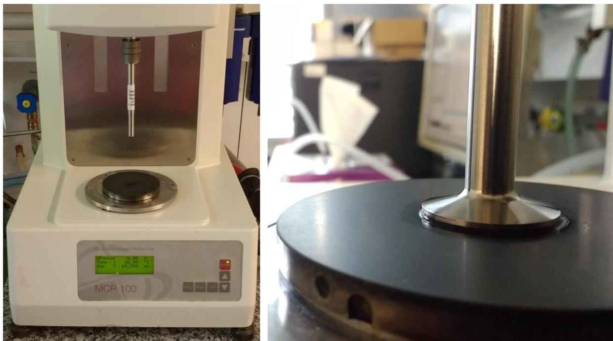
**Figure 2.7:** MCR 100 rheometer (left) with a PP25 measuring plate (right) used for bulk rheology measurements.
