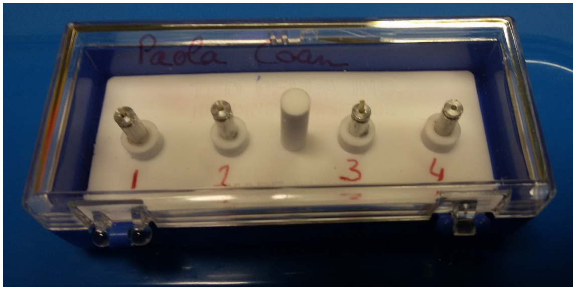
Figure 4.2 Three samples prepared for imaging at ID16a; the samples are in the dimension of 0.5mm x 0.5mm x 3mm (width x depth x height), samples are decalcified and fixed in paraffin.
