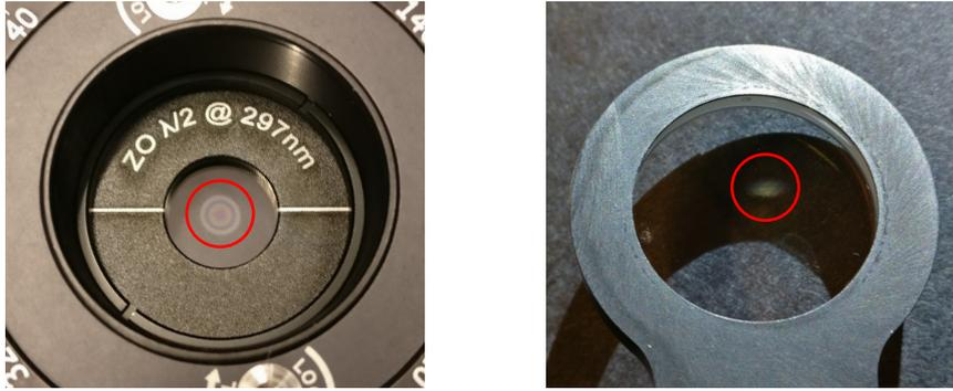
**Fig. 5.14** Damage and deposition of optical elements due to UV light. Damaged wave plate (**left**) and coated beam sampler (**right**). The opaque layer can be removed by cleaning with isopropanol and acetone, indicating a surface contamination.
