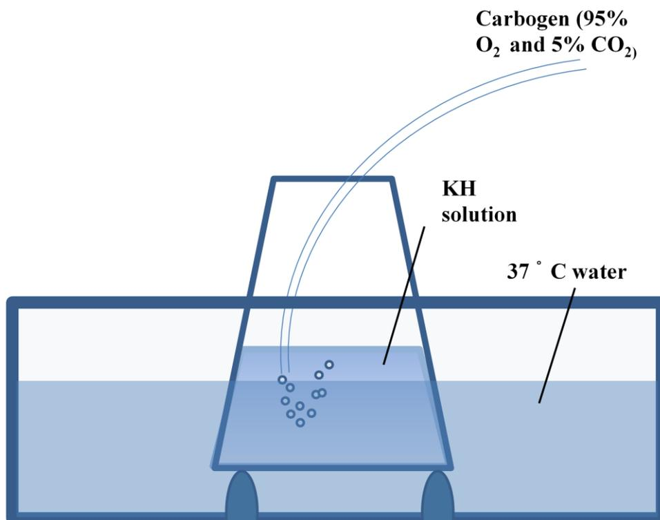
**Figure 6. The KH solution in a water bath and under carbogen inflow.**
