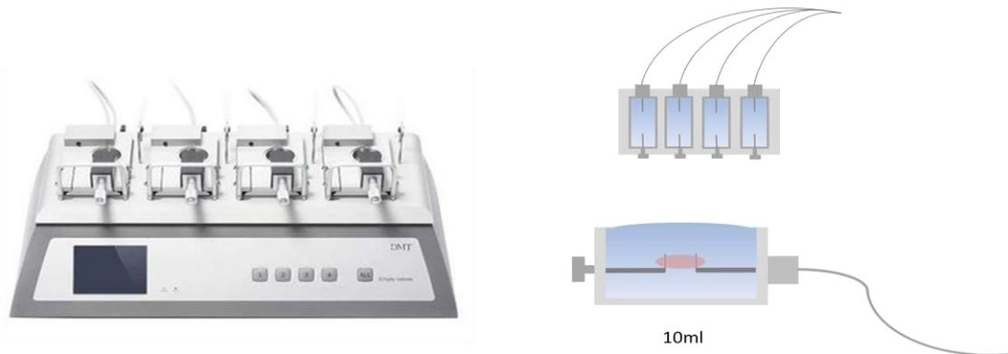
**Figure 7. The myograph machine and strips in the organ bath chambers.** A myograph device contains 4 chambers. Each chamber has a capacity of 10 ml liquid, with a independent adjustment knob and a force transducer.
