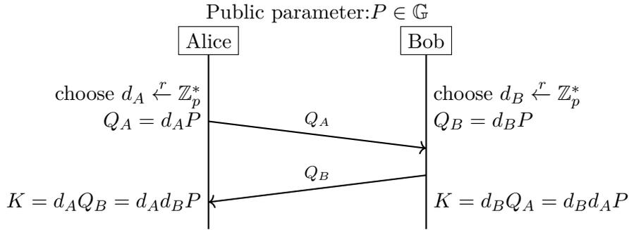
Figure 3.2: Elliptic Curve Diffie-Hellman (ECDH).
