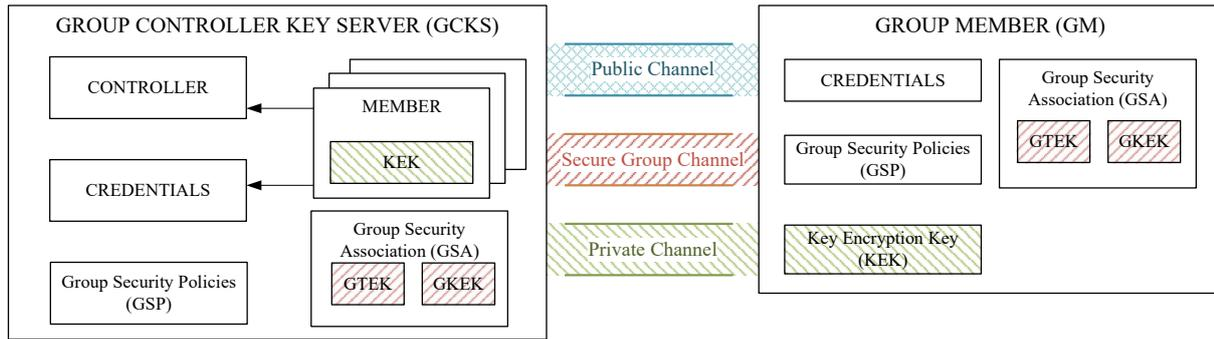
Figure 3.3: Group key management architecture as in RFC 2093 [116] and RFC 2094 [117].
