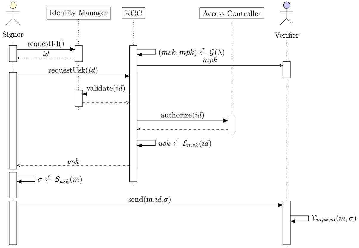
Figure 4.2: Communication model for IBS.
