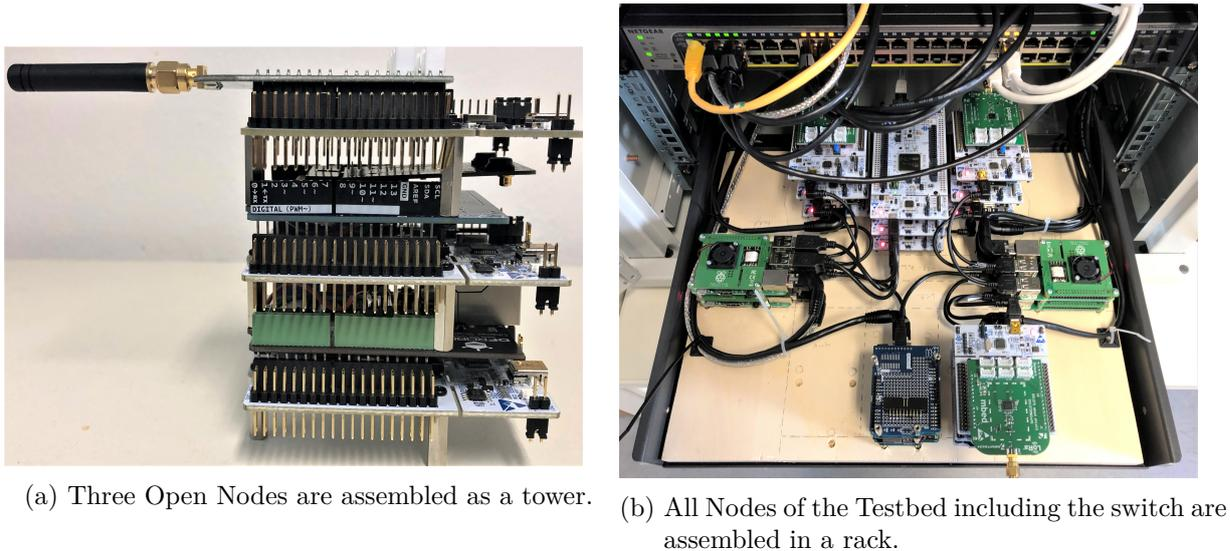
Figure 6.3: The installation of the testbed.
