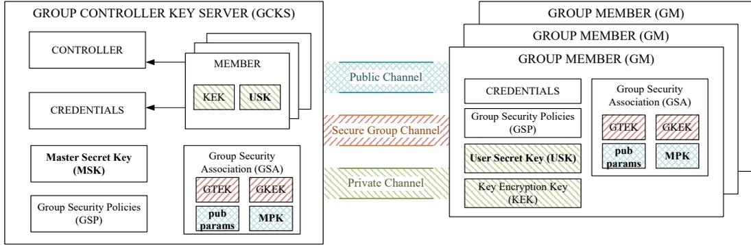
Figure 4.1: IBS key management within a group key management architecture described in RFC 2093 [116] and RFC 2094 [117]. Bold elements are IBS specific.
