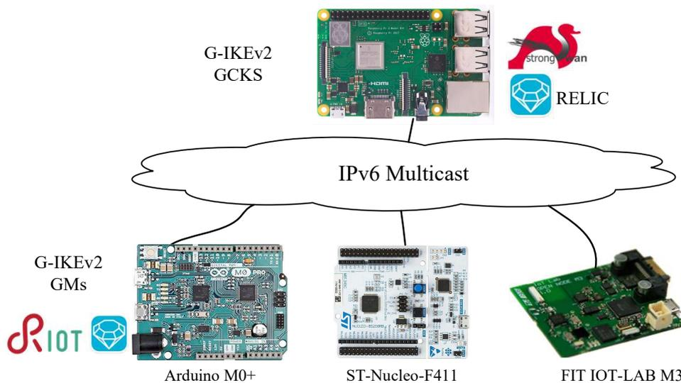
Figure 6.4: Implementation of a gIBS system with G-IKEv2 on the testbed.
