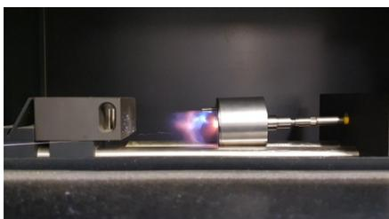
**Figure A5.17** Moment of detonation during the positive laser initiation test of complex **12**.
