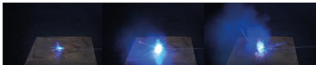
**Figure A5.16** HN of complex **12**. Moment of deflagration shown as a sequence.
