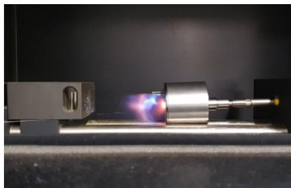
**Figure 5.13** Moment of detonation during the positive laser initiation test of complex **12**.
