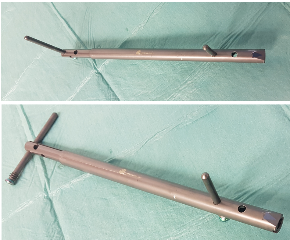
● Fig.16 The crown breakage caused instability of the anti-rotation mechanism of the PRECICE® nail
