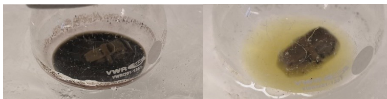
Figure 12: Titration of KDA (a) base before titration; (b) titration mixture after reaching the endpoint.
