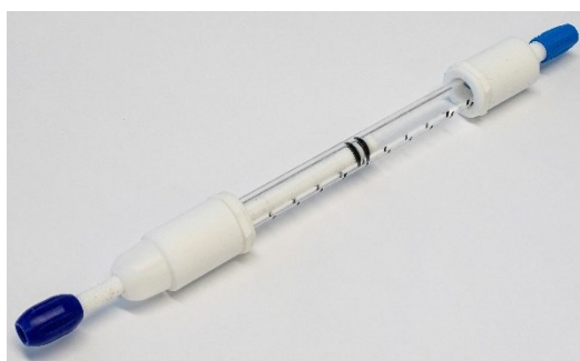
Figure 7: Glass column for the precise packing of a packed-bed reactor with various solids or heterogeneous catalysts.
