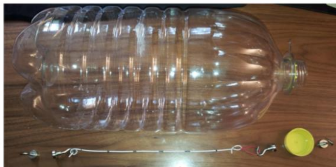
Fig. 1 A container was filled with water at body temperature (36 °C). Stents were fixed with clips at both ends and spanned throughout the phantom model for measurements
