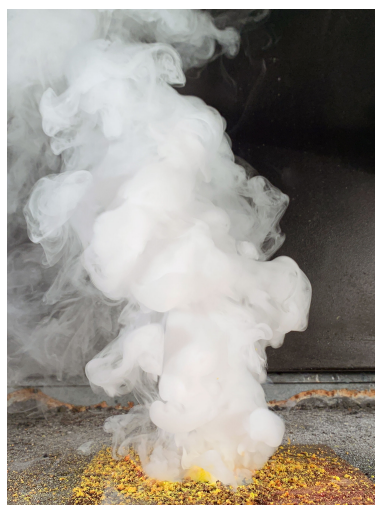
Figure 4.4: Guanidinium 5,5’-azotetrazolate as white smoke generator.
