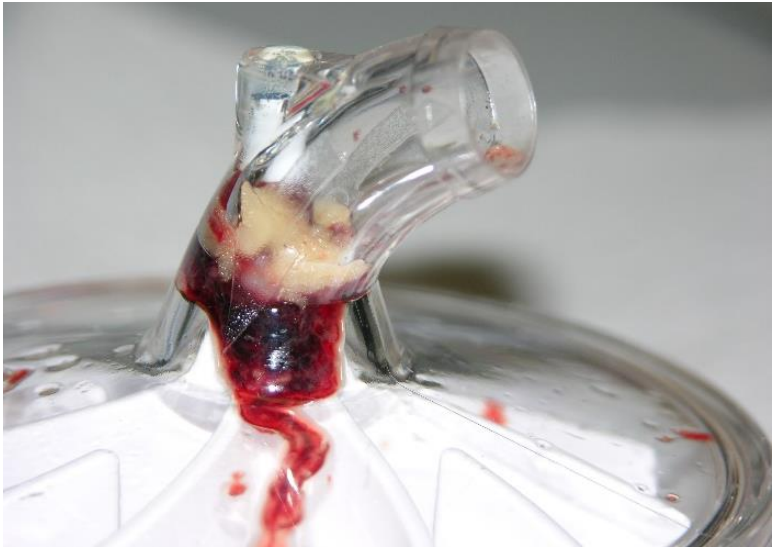
Abbildung 24: Thrombus in Pumpenkopf
