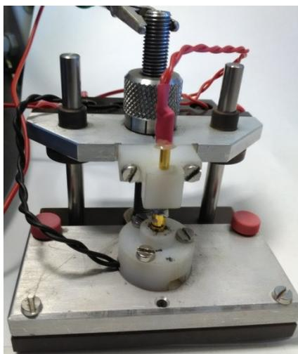
Figure S23 **In-house constructed dc-conductivity measurements cell for low sample volumes. Catalyst powder sample loosely compressed by opposing brass cylinder electrodes. Contact area of electrodes 0.126 cm<sup>2</sup>.**
