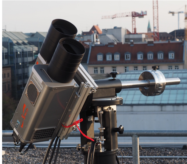
Figure 3.3: specMACS VNIR and SWIR sensors on the roof of the meteorological institute in Munich (Ewald et al., 2016)
