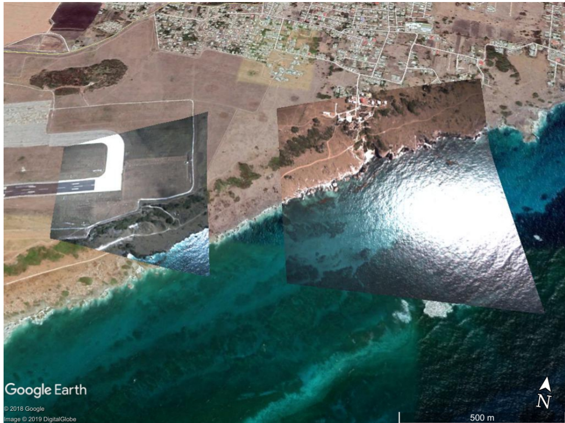
Figure 3.11: An example for the finished alignment procedure of the 2D camera during takeoff at the Grantley Adams International Airport on Barbados: the images have been aligned according to the procedure described in Section 3.3.1, both using the same final mounttree. The left image has been projected using the runway elevation as terrain height, while the right image has been projected using 0 (i.e. sea level) as terrain height. As there is a difference of about 50 m in elevation, only the runway or the shoreline match up in the reprojection respectively.
