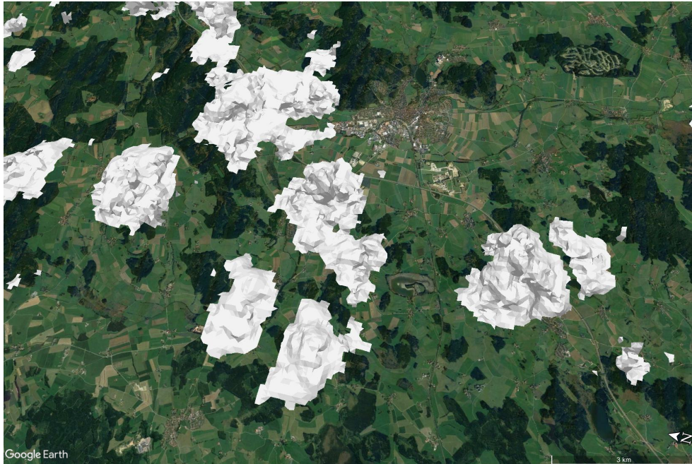
Figure 4.20: Reconstructed cloud surface: Cloud surface mesh, extracted via Poisson surface reconstruction from stereographically retrieved points (Fig. 4.19). The reconstructed cloud surfaces have been converted to a COLLADA (Barnes et al., 2008) model and geo-referenced using KML, such that the surfaces can be observed interactively using Google Earth. The perspective is roughly chosen to match the view of Figure 4.18.
