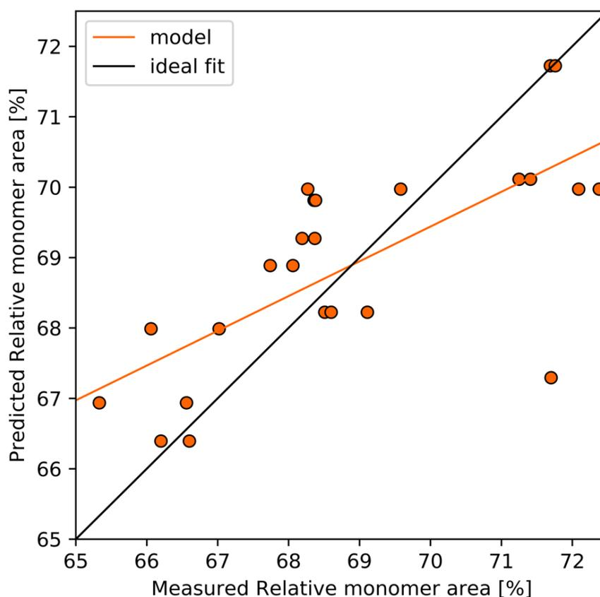
Figure 6.6: Multiple regression model to predict the effect of a small molecule on the relative monomer area determined by the ReFold assay.  $R^2=0.49$ ,  $RMSE=2.13$ .
