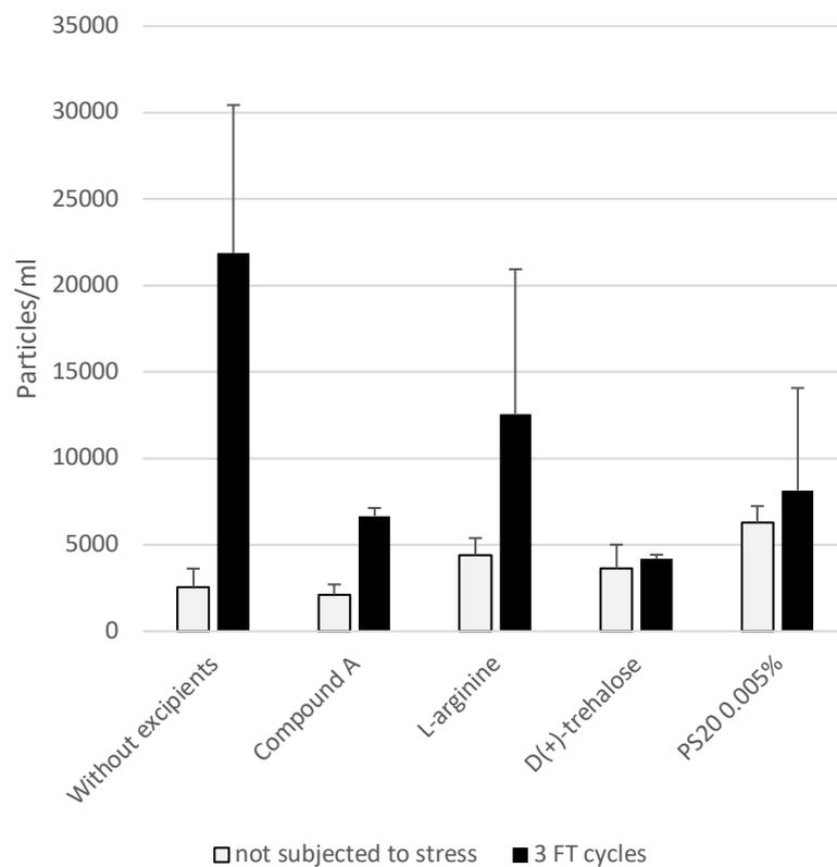
Figure A 4: Number of particles after 3 freezing/thawing cycles. 50 mM phosphate buffer, pH 7.0; 1 mg/ml interferon-alpha-2a.
