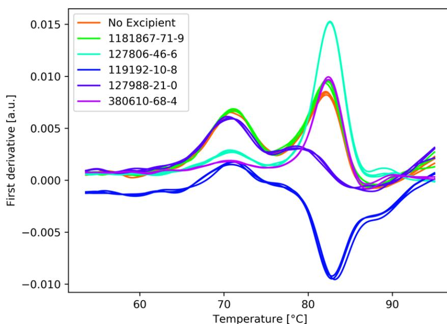
*Figure 6.5: First derivative of nanoDSF data for all ReFold stabilizers. All compounds except 1181867-71-9 significantly alter the shape of the curve in the transition region (n=3).*
