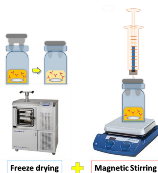
Figure 5-1 Scheme of mAb loaded VPG formulation storage by freeze-drying and reconstitution with magnetic stirring method.
