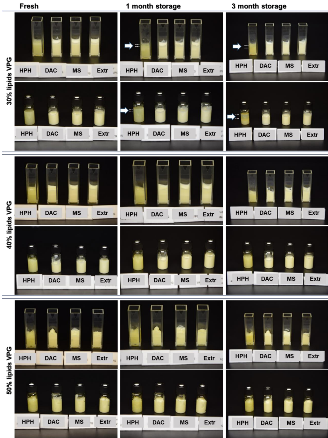
Figure 6-7 The appearance of VPGs from different preparation methods after scale-up manufacture during the storage study. The 30%, 40%, and 50% lipid content VPGs were prepared by different methods, and stored for 1 month, and 3 months.
