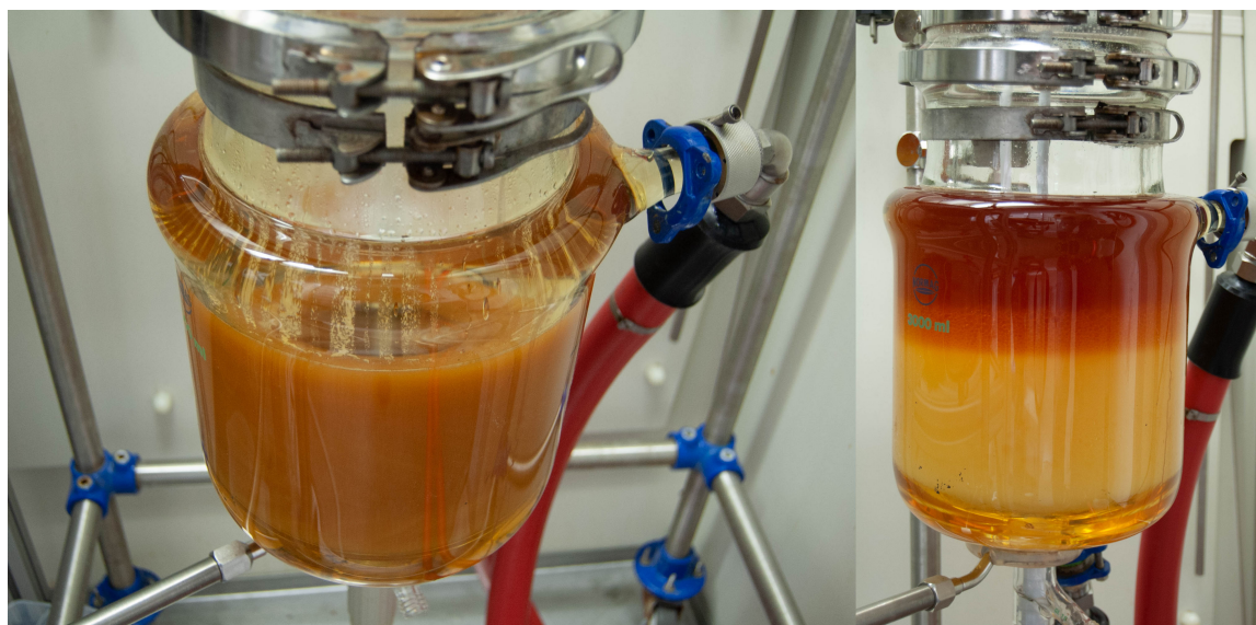
Figure 6.7 Azidation setup for experiments CAP1 and CAP2 . 3 L double-jacket reactor equipped with KPG stirrer connected to a Huber unistat. Left picture was taken during the reaction, the right picture shows the phase separation during the first extracting step after quenching.
