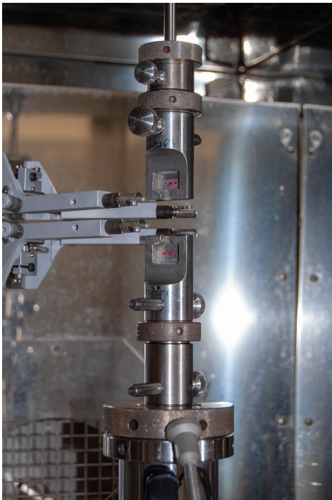
Figure 4.2 Zwick UPM 1476 tensile test machine at Fraunhofer ICT. Setup in a thermo-chamber, which can be operated in a temperature range between −40 °C and 60 °C.
