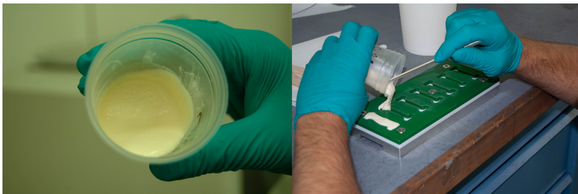
Figure 7.17 Propellant slurry after addition of all ingredients (left). Casting process of the propellant slurry into the molds for tensile test specimen (right).
