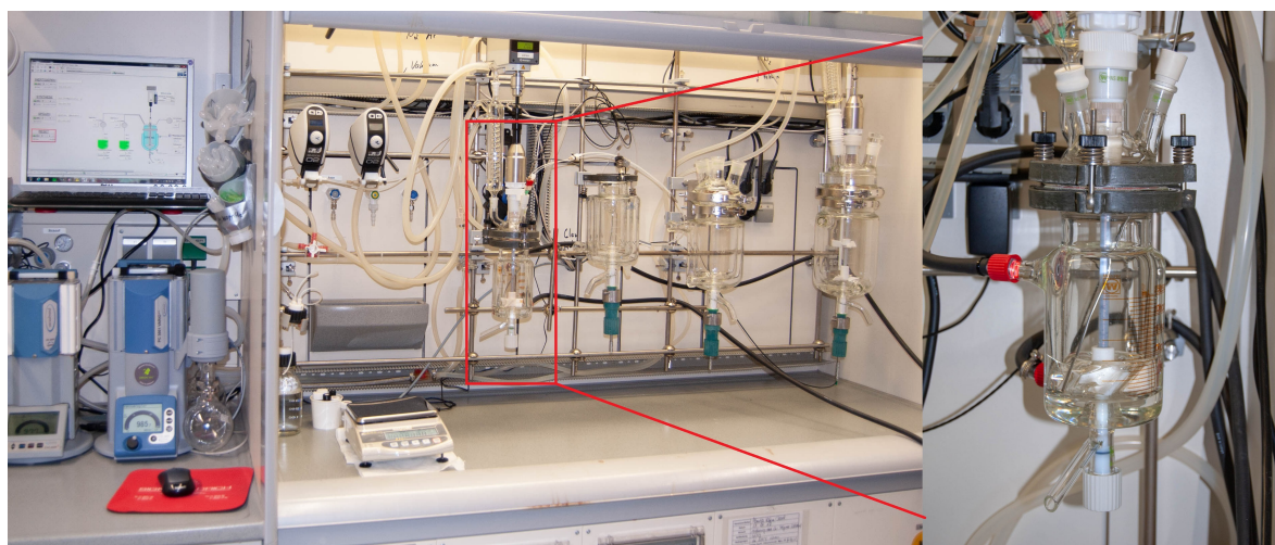
Figure 6.2 Setup for polymerization scale-up experiments. A 250 ml double-jacket reactor with magnetic stirring coupling was connected to a HiTec Zang reaction automation system.
