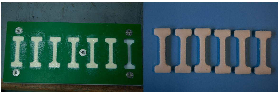
Figure 7.18 Tensile test specimen before (left) and after demolding (right).
