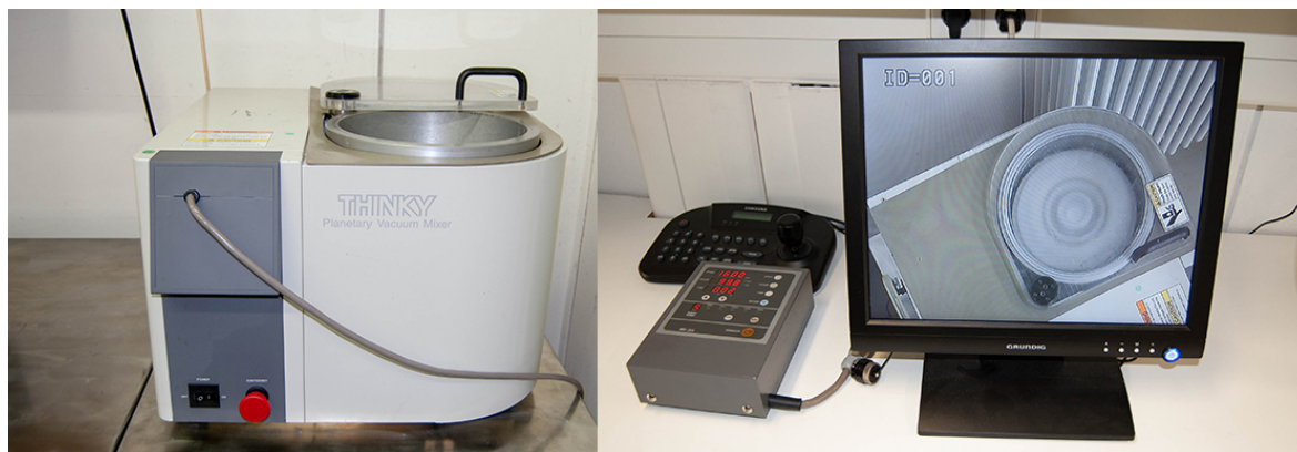
Figure 7.16 Mixing principle of the Thinky Mixer ARV-310. Device is operated safely under remote control [212].
