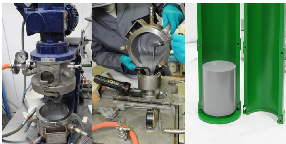
Figure 7.8 Processing of a small-scale propellant grain (end burner \approx 350 g) at Fraunhofer ICT. From left to right: mixing, casting and the final cured propellant grain.
