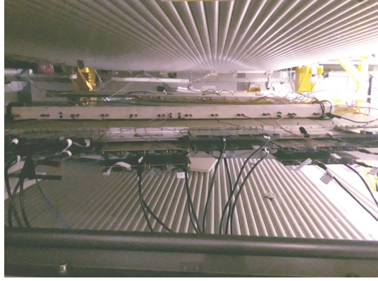
(b) Picture of a Micromegas module between the MDT chambers. The strips of the module are oriented parallel to the tubes of the reference chambers. On top of the module high voltage distribution boxes are situated. The readout electronics are attached at both tapered sides of the module.
