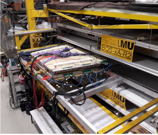
(a) Picture of the Cosmic Ray Facility in Garching near Munich. A Micromegas module is prepared for data-taking with black HDMI-cables and red high-voltage cables. The modules are placed on a support structure, which can be moved between the MDT chambers.
