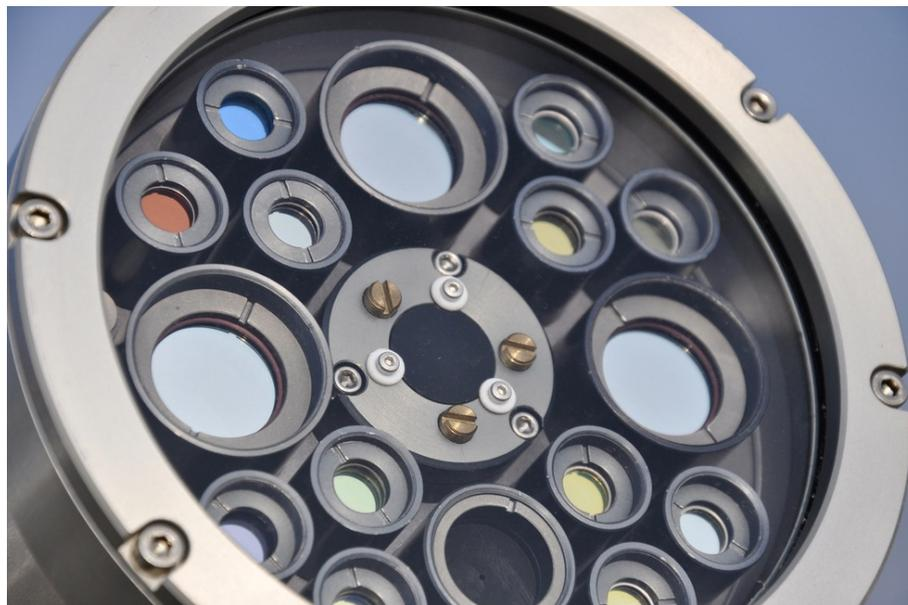
**Figure 3.1.:** SSARA sensorhead with 12 direct channels (smaller diameter tubes), and 3 polarized channels (larger diameter at the top, left and right). The quadrant sun-tracker is in the center, below it is a finder for manual sun tracking.
