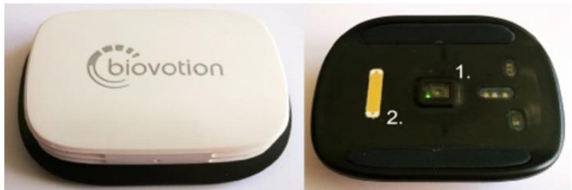
Figure 1. The Biovotion vital sign monitor (vsm-1). The sensors of the vsm-1 include an optical sensor (1), an acceleration sensor, a temperature sensor and a sweat sensor (2).
