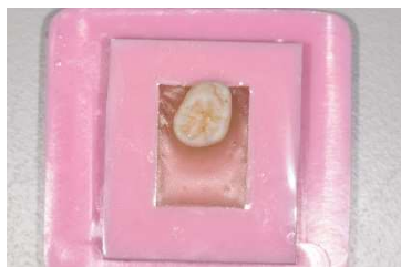
Technovitblock in Silikonform
