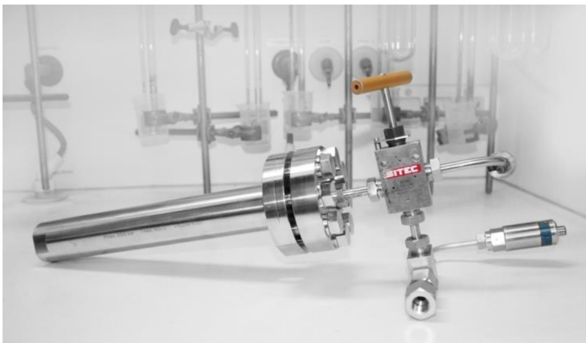
Figure 6. Custom-built autoclave made from Inconel 718 with peripheral equipment.
