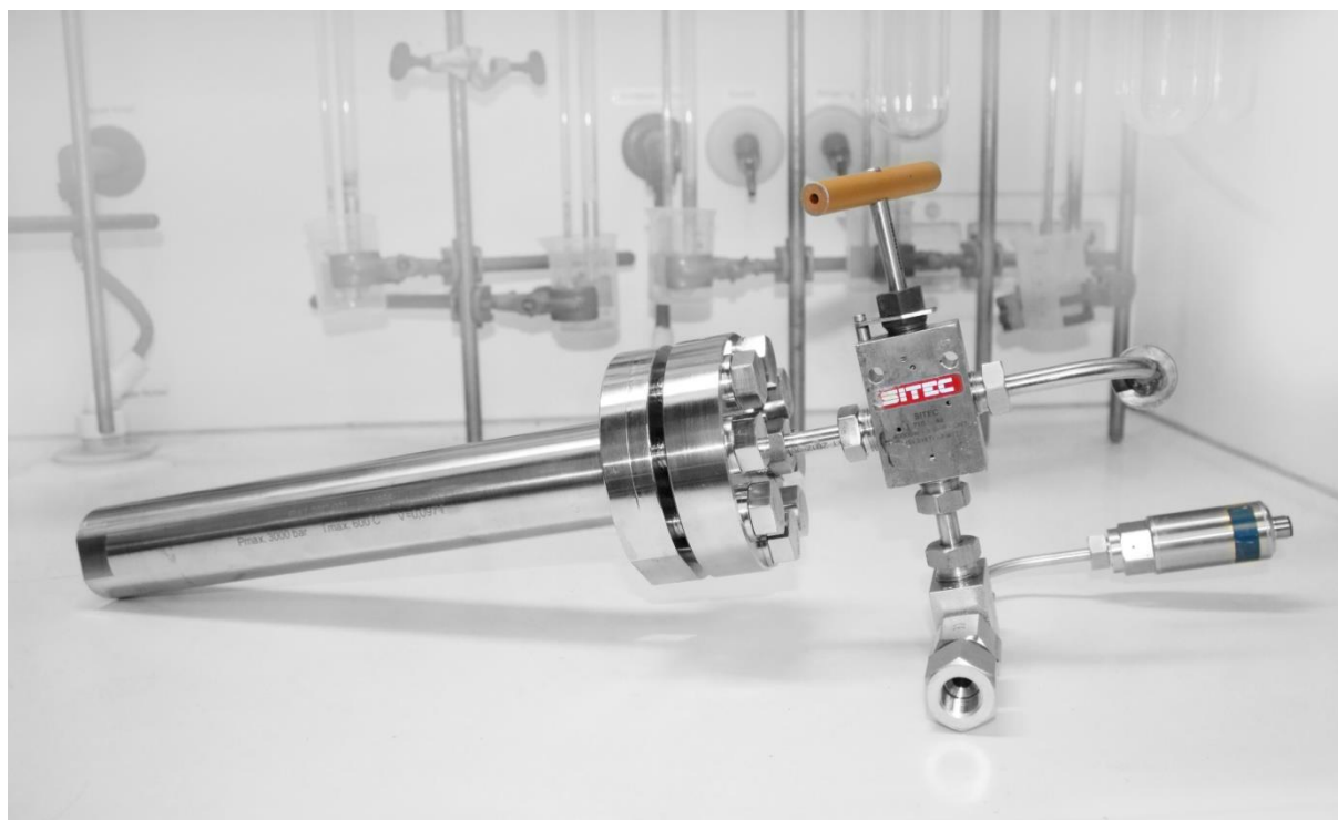
Figure 1: Custom-built autoclave made from Inconel 718 with peripheral equipment.
