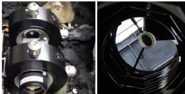
Figure F.5: Left: Mouse using front-end part of the receiver as burrow. Right: scratches on the Newtonian telescope’s primary mirror.
