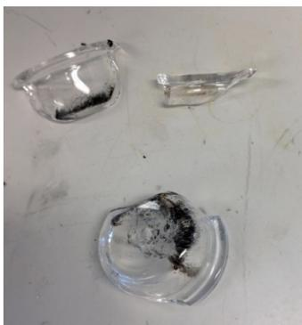
Figure 6.2: Broken fused quartz crucible.
