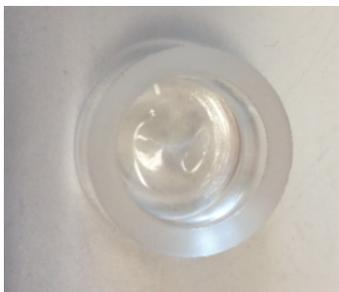
Figure 6.3: Stable fused quartz crucible.
