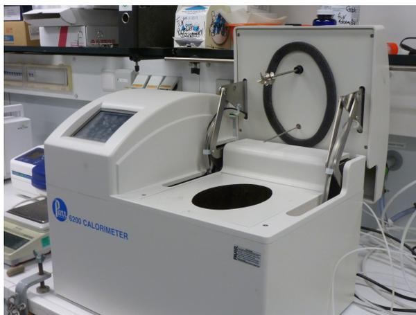
Figure 4.2: 6200 Isoperibol oxygen bomb calorimeter.
