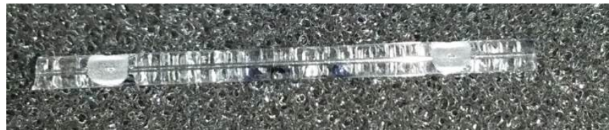
(d) Fiber with drilling holes for gas access.
