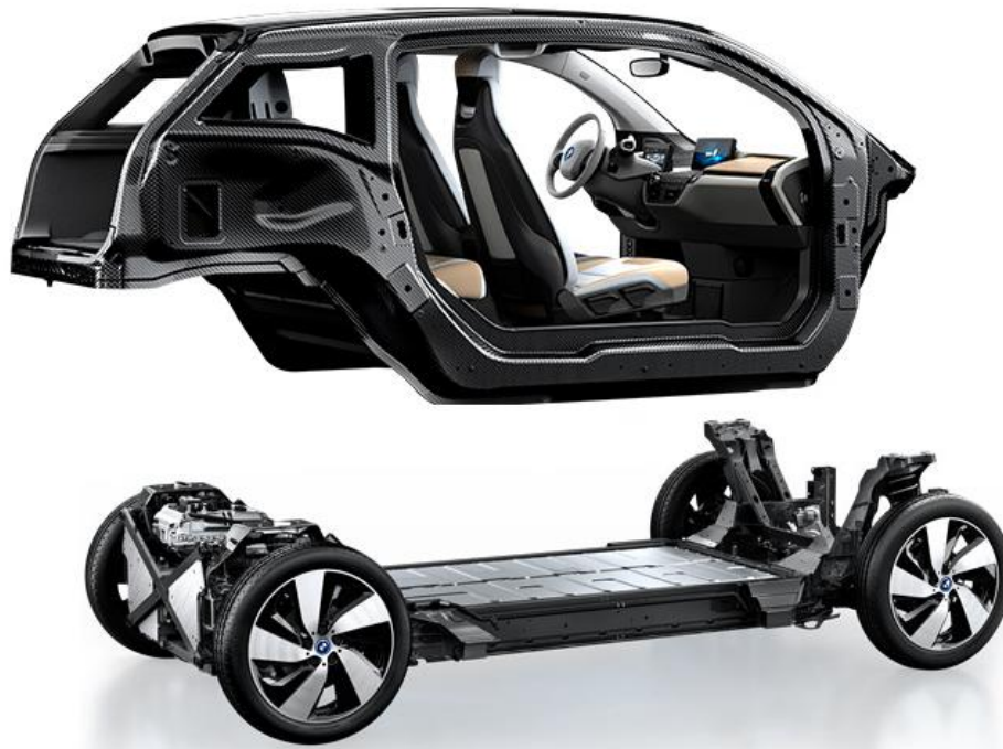
Figure 1: BMW LifeDrive-Concept realized in BMW i3 with Life-Module (top) and Drive-Module (bottom). [5]
