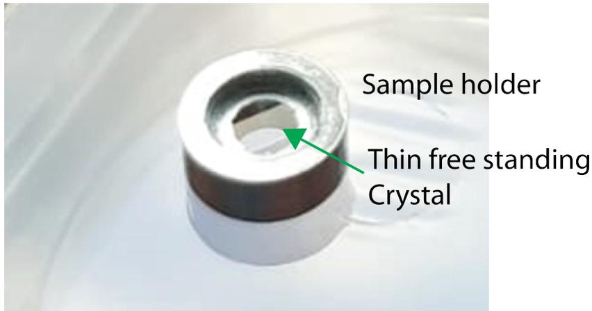
Figure 6.7:  $\text{MgF}_2$  crystal with  $5 \mu\text{m}$  thickness and 2 mm diameter mounted on an cylindrical frame.
