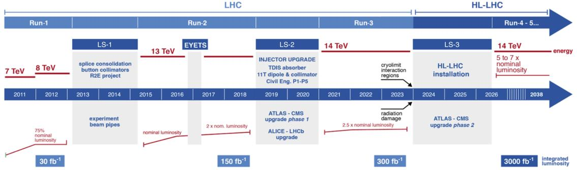
Figure 2.3: Schedule of LHC operations on the road to HL-LHC. The image is adapted from Reference [11].
