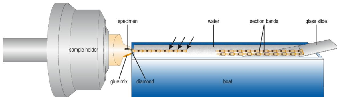
**Fig. 4.** Setup for semithin serial sectioning. The layer of glue mix on the ventral side of the specimen block ensures, that the following section is firmly attached to the previous section (arrows). Once several bands are attached to the glass slide, the slide is removed from the boat and dried.
