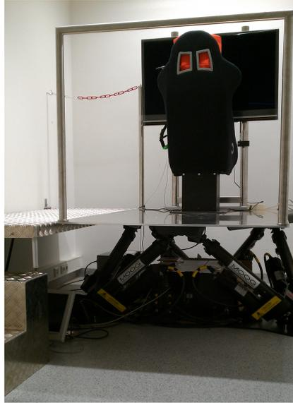
Figure 1.9: 6-degree-of-freedom hexapod motion platform
