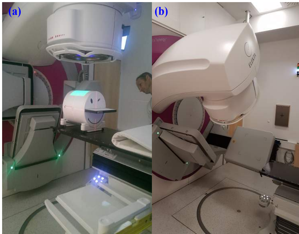
Figure 6.4: Picture of (a) Octavius setup (b) In-air image acquisition of EPID during a plan delivery.
