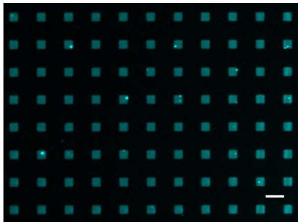
Figure 2.8: IgM antibody array generated with plasma-induced patterning. Squares with a side length of 25 \mu\text{m} are coated with an IgM anti-CD15 antibody and the backfilling (black) area with PLL-g-PEG(2kDa). For visualising the IgM coated squares a goat anti-mouse secondary antibody conjugated with AlexaFluor488® was used, the surface was blocked with 5% w/v nonfat dry milk. The image was acquired with a 10x objective, and the scale bar corresponds to 60 \mu\text{m} .
